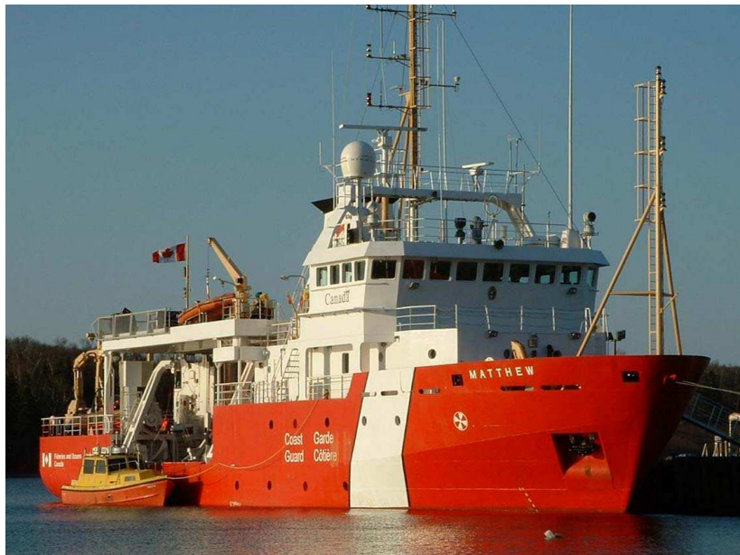
Figure 1. Multibeam bathymetry and sub-bottom profiler data were collected using the CCGS Matthew equipped with a Kongsberg EM710 multibeam bathymetry system and one hydrographic launch equipped with a Kongsberg EM3002 multibeam bathymetry system. Photo courtesy of J. Shaw.
