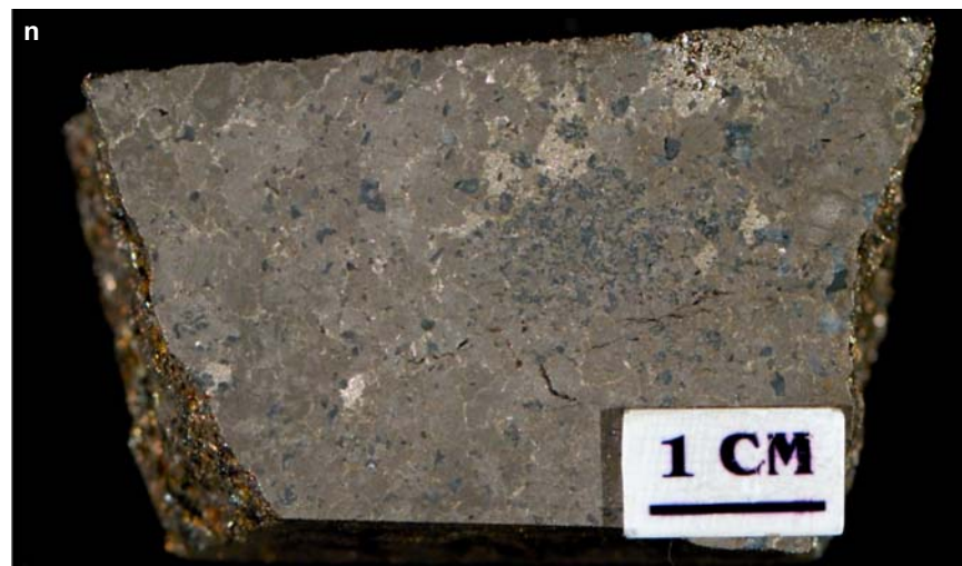
Figure SR2.1n. Creighton mine. Massive pyrrhotite-pentlandite with minor chalcopyrite (1.6% Cu, 5.7% Ni). Sample 98-AV-38, 7400 level- 6635D.
