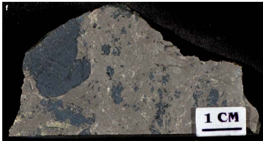
Figure SR1.12f. Victoria Embayment. Sheared massive pyrrhotite with interstitial pentlandite and minor chalcopyrite and porphyroclasts of altered host rock. Sample 98-AV-87, collected in 1918 by H.V. Ellsworth from Lot 8, Con 2, Denison Township.
