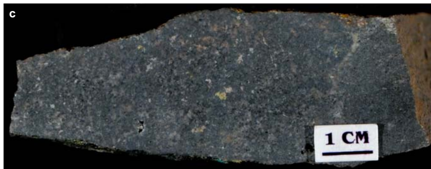
Figure SR3.7c. Vermillion mine. 5% disseminated bornite-chalcopyrite in quartz diorite. Sample 00AV-507.
