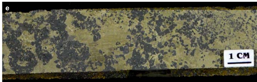
Figure SR2.2e. Segway deposit. Massive coarse chalcopyrite-magnetite-pyrrhotite. Sample 05AV-16, bore hole FNX8001, 222.3 ft.
