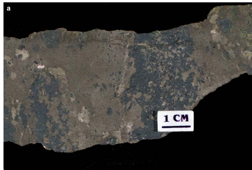
Figure SR5.2a. Falconbridge mine. Semi-massive pyrrhotite with blebby pentlandite and disseminated chalcopryite stringers. Sample 98-AV-67.
