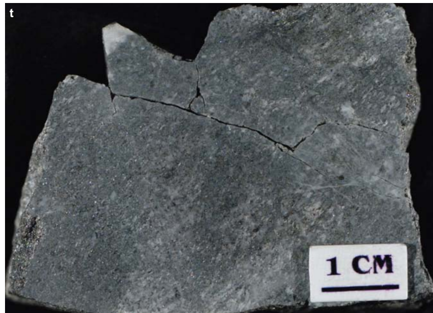
Figure SR1.4t. Creighton mine. Disseminated sulphide in sheared, possibly sedimentary, biotite-quartz rock. Sample 02-AV-657, 5900 level 4930 drift 4030B.
