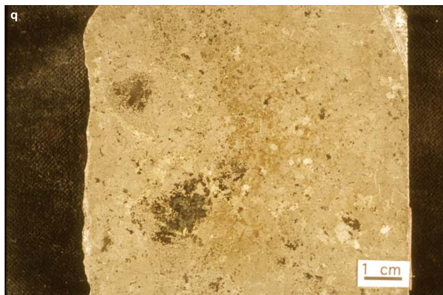
Figure SR1.3q. Crean Hill deposit. Representative massive pyrrhotite-pentlandite-chalcopyrite-magnetite. Sample CH-6, Inco collection, collected between approximately 1996 and 1971.
