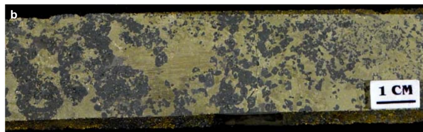
Figure SR2.2b. Segway deposit. Massive coarse chalcopyrite with coarse blebby magnetite and minor coarse pyrrhotite. Sample 05AV-14, bore hole FNX8001, 208.7 ft.
