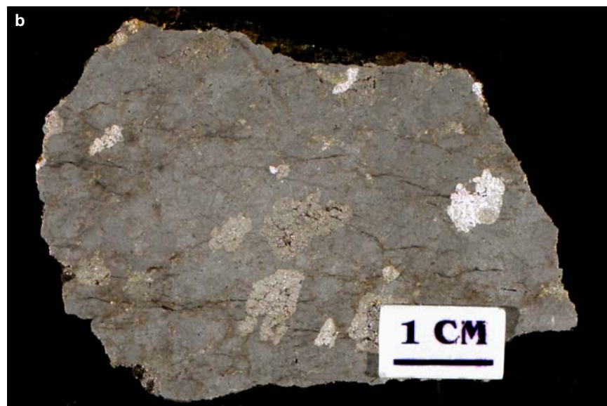
Figure SR1.3b. Crean Hill deposit. Massive pyrrhotite with blebby pentlandite. Sample 98-AV-46, 2800 level 2800B.
