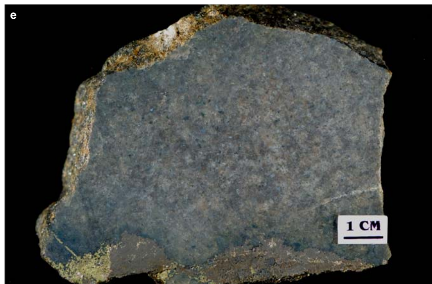
Figure SR1.10e. Murray mine. Massive pyrrhotite vein with minor chalcopyrite-magnetite cross-cutting Footwall granite. Sample EI-70-05, collected by Roger Eckstrand from the 1650 level.
