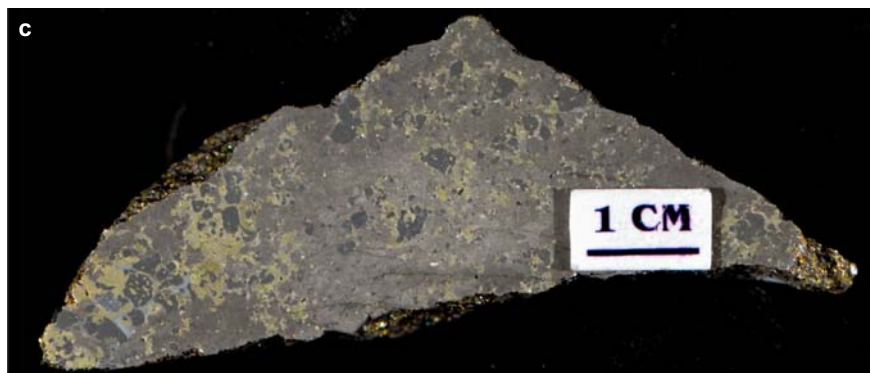
Figure SR3.9c. Worthington mine. Massive pyrrhotite with disseminated chalcopyrite stringers and 20% disseminated magnetite blebs. Sample 98-AV-62, collected in 1900 by H.V. Ellsworth from Lot 2, Con 1, Drury Township.
