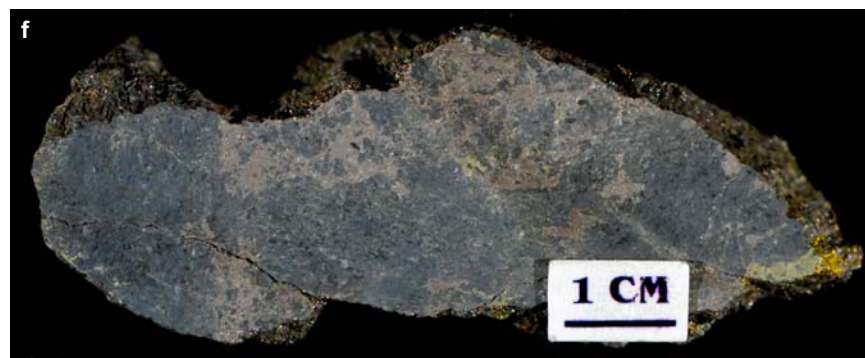
Figure SR1.3f. Crean Hill deposit. Semi-massive chalcopyrite vein. Sample 98-AV-50, 3840 level 3840B.
