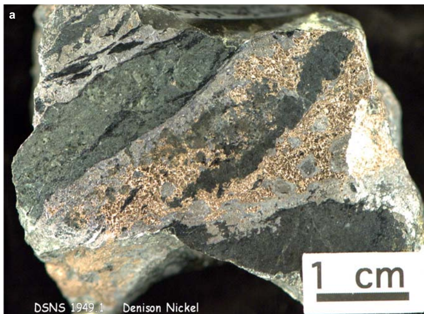
Figure SR3.2a. Denison Township. 50% niccolite-gersdorffite>chalcopyrite in mafic-ultramafic rock with quartz veins. Gersdorffite forms 3 to 4 mm cubes. Sample DNSN1949-1, collected in 1949 by W.C. Ringsleben from Lot 8 Con X1.
