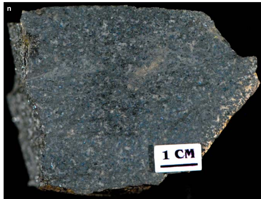
Figure SR3.1n. Copper Cliff deposit. 1% disseminated pyrrhotite-chalcopyrite in sheared quartz diorite. Sample EI-70-07, collected by Roger Eckstrand from a surface outcrop.
