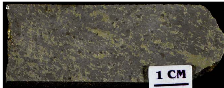
Figure SR2.2a. Segway deposit. Massive coarse pyrrhotite with interstitial chalcopyrite and finely disseminated magnetite. Sample 05AV-13, bore hole FNX8001, 207 ft.
