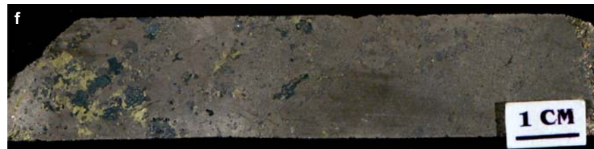
Figure SR2.2f. Segway deposit. Massive coarse pyrrhotite with blebby magnetite-chalcopyrite. Sample 05AV-18, bore hole FNX8001, 229 ft.
