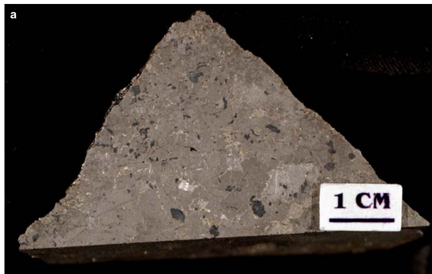
Figure SR1.3a. Crean Hill deposit. Massive pyrrhotite with blebby pentlandite and disseminated chalcopyrite and small mafic fragments. Sample 98-AV-45, 2800 level 2800A.
