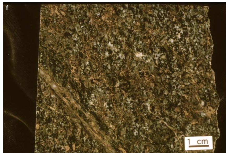
Figure SR1.6f. West Kirkwood mine. Typical ore with 15% blebby to stringer pyrrhotite-chalcopyrite in coarse-grained diorite. Sample K-7, Inco collection.
