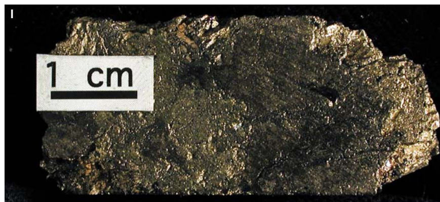
Figure SR3.6l. Totten deposit. Massive pentlandite. Sample 01-AV-252.
