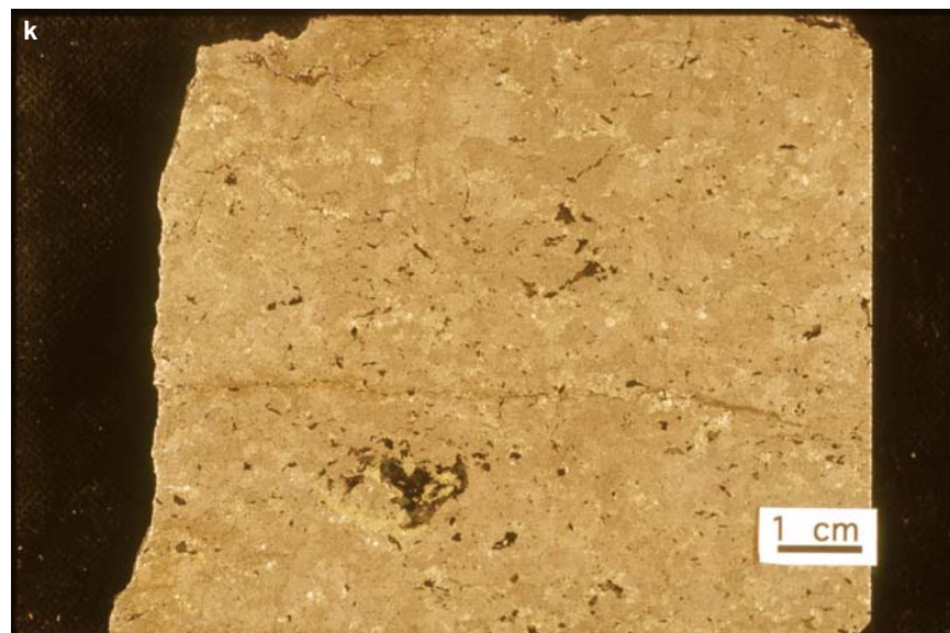
Figure SR1.2k. Clarabelle deposit. Representative massive sulphide composed of pyrrhotite-pentlandite-chalcopyrite and bornite. Sample CL-11, Inco collection.
