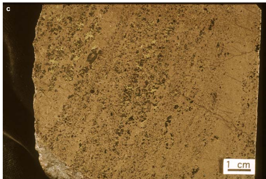
Figure SR1.6c. Main Kirkwood mine. Representative massive pyrrhotite-chalcopyrite-magnetite ore. Sample K-3, Inco collection.
