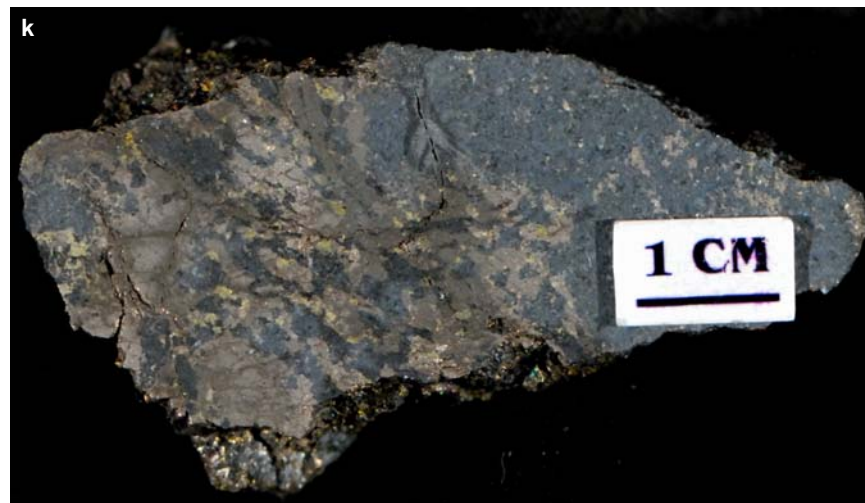
Figure SR4.2k. Frood-Stobie mine. Interstitial to semi-massive pyrrhotite-chalcocopyrite within mafic rock. Sample 98-AV-76, collected by Rod Kirkham from the Frood-Stobie pit.
