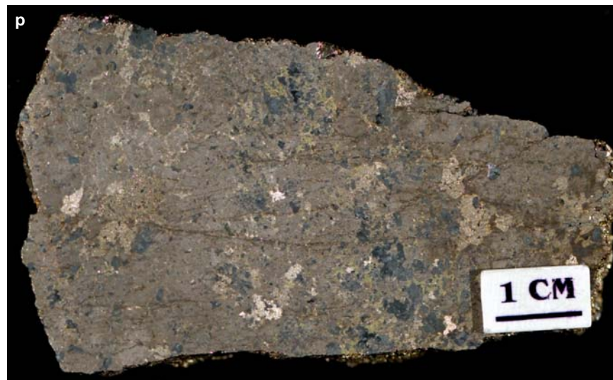
Figure SR2.1p. Creighton mine. Massive pyrrhotite with blebby pentlandite and disseminated chalcopyrite (1.8% Cu, 6.9% Ni). Sample 98-AV-40, 7400 level - 6545D.
