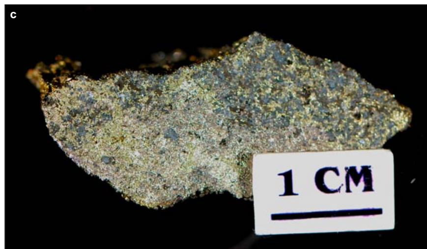
Figure SR2.1c. Creighton mine. Semi-massive chalcopyrite-pyrite-millerite(?) in quartz diorite. Sample EI-74-312, collected by Roger Eckstrand from the 5800 level, 403 orebody.
