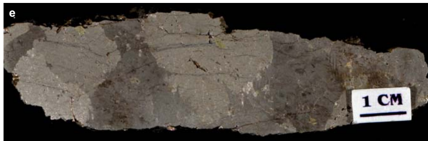
Figure SR3.9e. Worthington mine. Massive pyrrhotite-pentlandite with minor chalcopyrite. Note 2 cm pentlandite crystals. Sample 98-AV-64, collected in 1918 by H.V. Ellsworth from Lot 2, Con 2, Drury Township.
