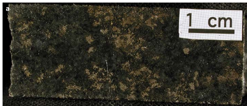
Figure SR1.1a. Blezard deposit. 30% interstitial pyrrhotite-pentlandite in gabbro. Sample 01-AV-225A.
