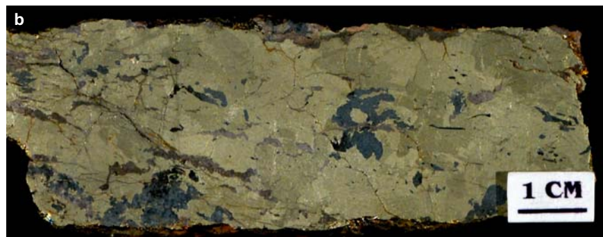
Figure SR1.12b. Victoria Embayment. Massive chalcopyrite-cubanite-pyrrhotite-bornite, mineralized amphibolite inclusion surrounded by massive sulphide. Sample 00AV-510, Pit 2.
