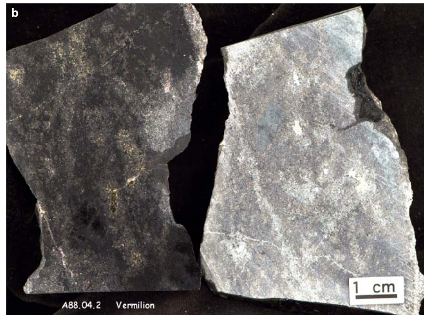
Figure SR1.11b. Vermillion mine. 20% disseminated chalcopyrite-PGM, very PGE-rich minerals, niccolite-violarite-gersdorffite-maucherite, polydymite in fine-grained chloritized quartz diorite. Sample A88-04-2A, collected in 1988 by H.G. Ansell from Denison Township.
