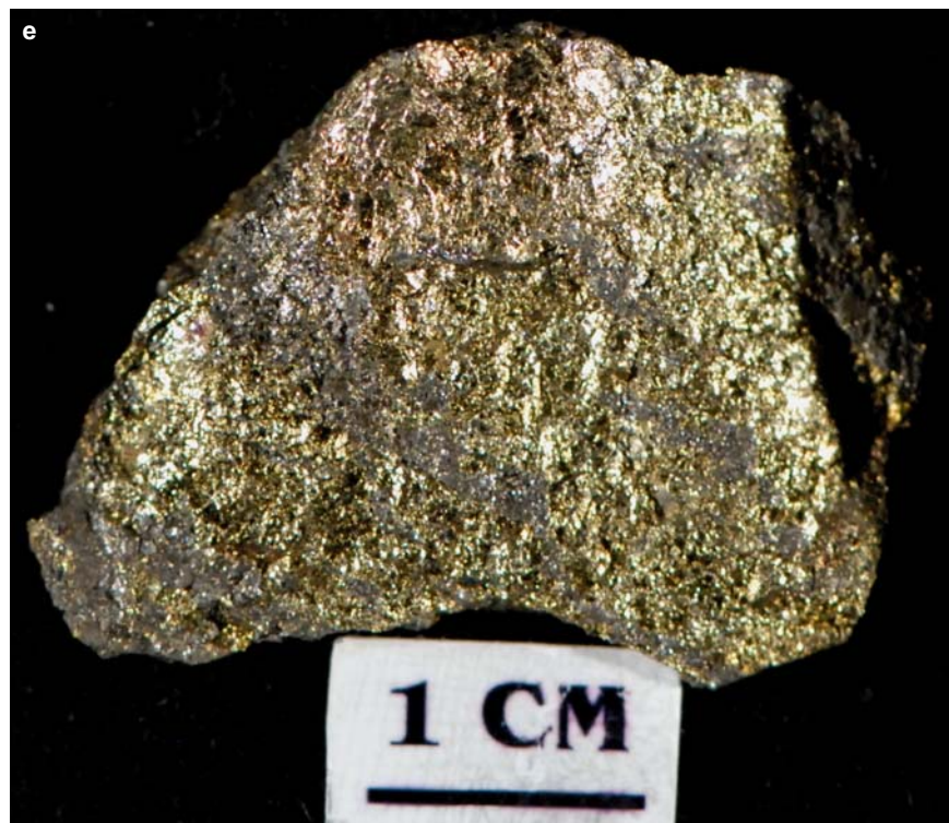
Figure SR3.1e. Copper Cliff deposit. Banded massive chalcopyrite- pyrrhotite, "tiger striped" with banded pyrrhotite within chalcopyrite. Sample 98-AV-90, collected in 1887 by R.C. Van Horne from Lot 12, Con 2, McKim Township.
