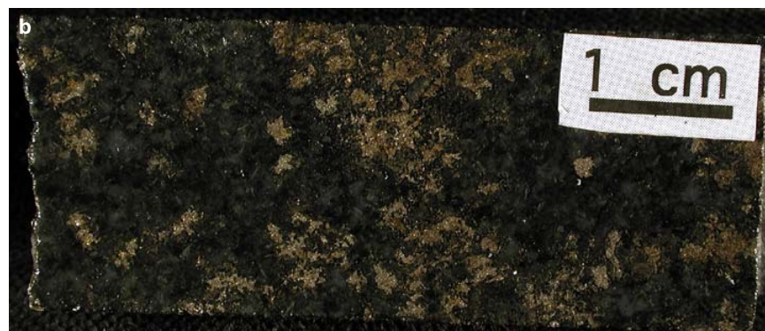
Figure SR1.1b. Blezard deposit. 30% interstitial pyrrhotite-pentlandite in gabbro. Sample 01-AV-225B.
