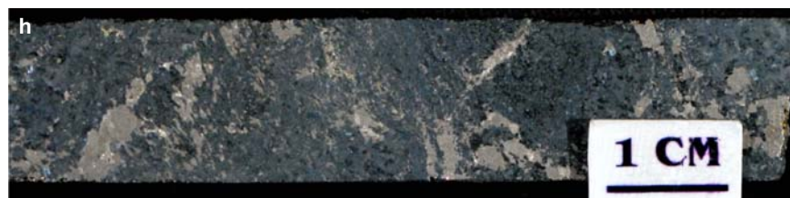
Figure SR3.1f. Copper Cliff deposit. Semi-massive pyrrhotite-chalcopyrite-pentlandite. Sample 98-AV-56, bore hole 100506, 312-312.5 ft, 100 orebody.
