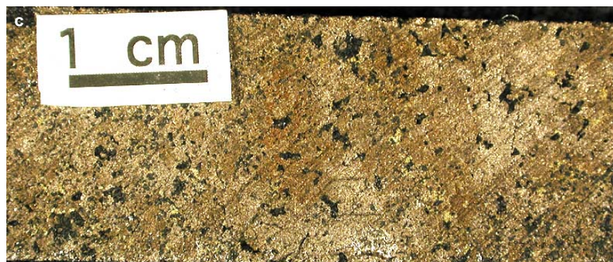
Figure SR1.1c. Blezard deposit. Massive pyrrhotite-pentlandite-bornite. Sample 01-AV-226.
