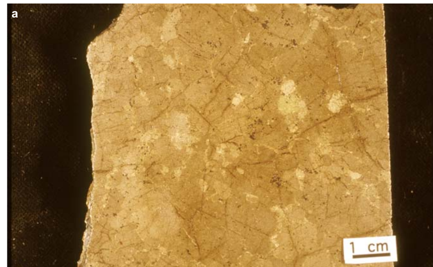
Figure SR1.2a. Clarabelle deposit. Representative contact massive sulphide composed of coarse pyrrhotite with pentlandite-chalcopyrite-magnetite. Sample CL-1, Inco collection, Creighton funnel.
