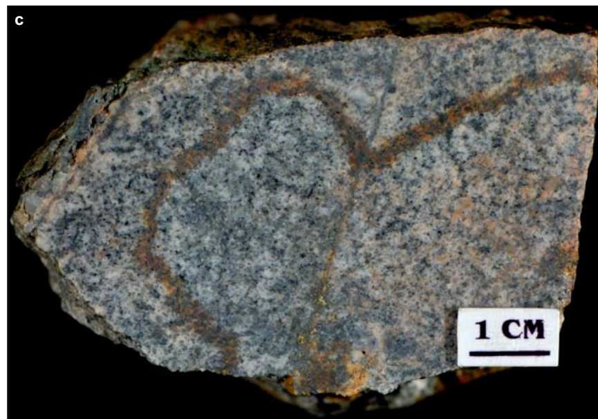
Figure SR3.8c. Victoria mine. 2% disseminated chalcopyrite-pyrrhotite within quartz diorite. Note aplite dyke cross-cuts quartz diorite, associated with shear zone. Sample 00AV-504.
