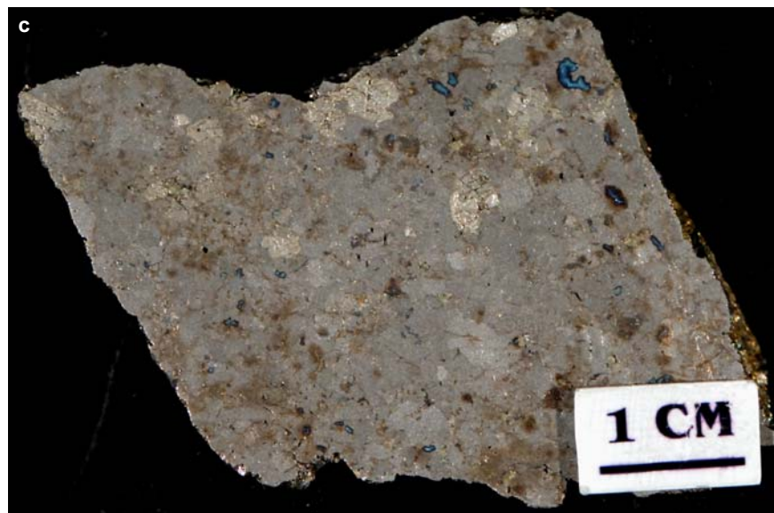
Figure SR1.3c. Crean Hill deposit. Massive pyrrhotite-marcasite with blebby pentlandite and disseminated chalcopyrite. Sample 98-AV-47, 3840 level 3840C.
