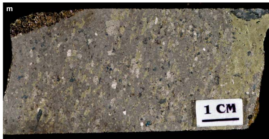
Figure SR2.1m. Creighton mine. Massive pyrrhotite-pentlandite-chalcopyrite. Sample 98-AV-37, bore hole 93763-1040 ft.
