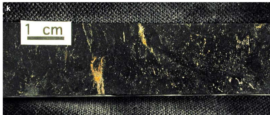
Figure SR1.1k. Blezard deposit. 2% disseminated pyrrhotite-pentlandite in fine-grained mafic rock. Sample 01-AV-235.
