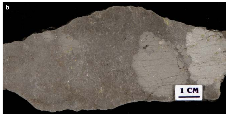
Figure SR3.9b. Worthington mine. Massive pyrrhotite-pentlandite with disseminated chalcopyrite blebs. Note large 2-3 cm pentlandite crystals. Sample 98-AV-61, collected by Barlow from Lot 2, R2, Drury Township.
