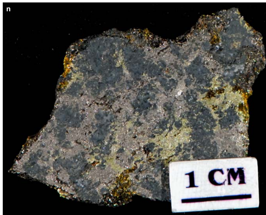
Figure SR4.2n. Frood-Stobie mine. Interstitial to semi-massive pyrrhotite-chalcopyrite in quartz diorite. Sample 98-AV-79, collected in 1929 from the 2400 level.
