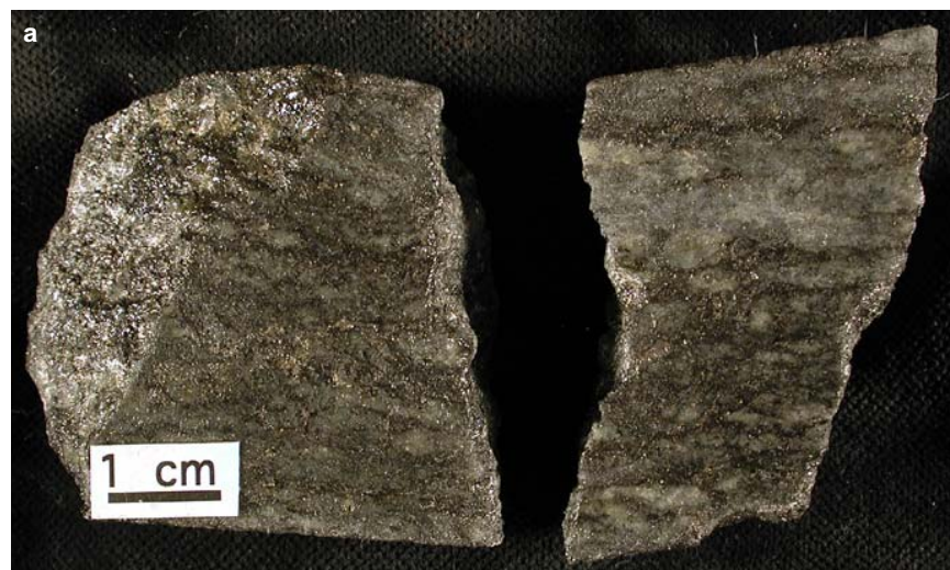
Figure SR3.6a. Totten deposit. 25% disseminated and banded silver-bearing sulphide mineral in epidote-altered quartz diorite(?). Sample 01-AV-241, RX#230292.
