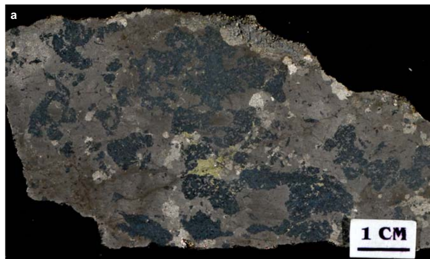
Figure SR3.3a. Evans mine. Semi-massive pyrrhotite-chalcopyrite-millerite. Sample 98-AV-80, collected by H.V. Ellsworth in 1929 from Lot 1, Con 1, Snider Township.
