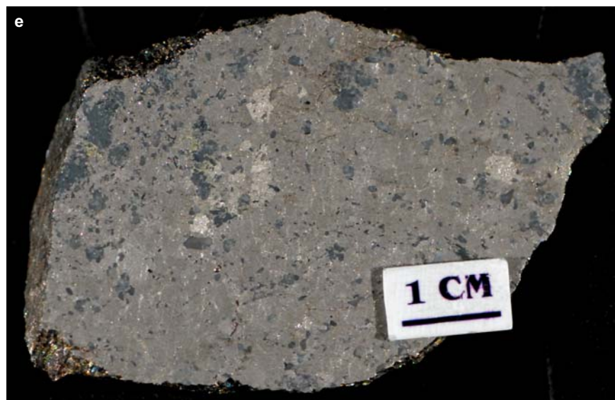
Figure SR1.3e. Crean Hill deposit. Massive marcasite with blebby pentlandite and disseminated chalcopyrite. Sample 98-AV-49, 3980 level 3980B.
