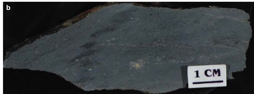
Figure SR3.7b. Vermillion mine. Chalcopyrite-rich stringer between two pods of quartz diorite. Sample 00AV-506.
