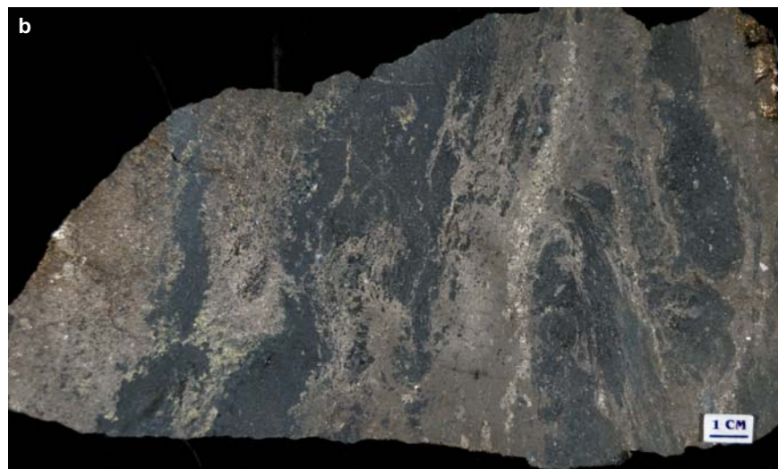
Figure SR5.2b. Falconbridge mine. Banded massive pyrrhotite with minor chalcopryite along scapolite vein (in mafic host rock?). Sample EI-70-15A, collected by Roger Eckstrand from the #5 zone, 4800 level.
