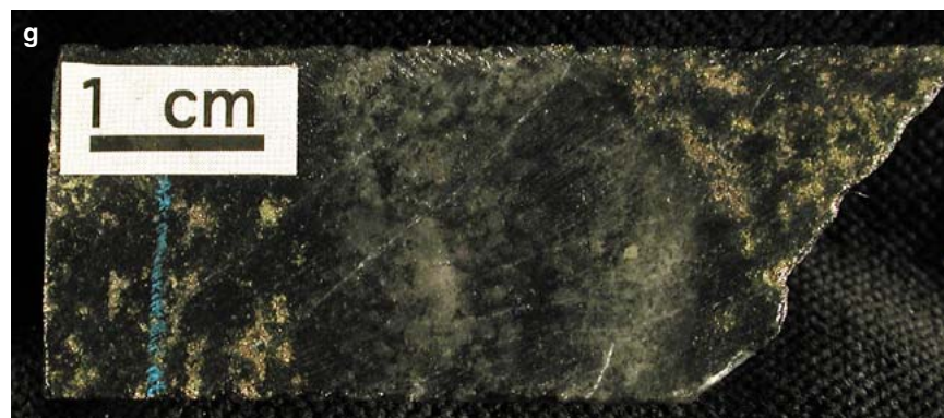
Figure SR3.6g. Totten deposit. 25% disseminated to interstitial pyrrhotite-chalcopyrite in breccia. Sample 01-AV-247.
