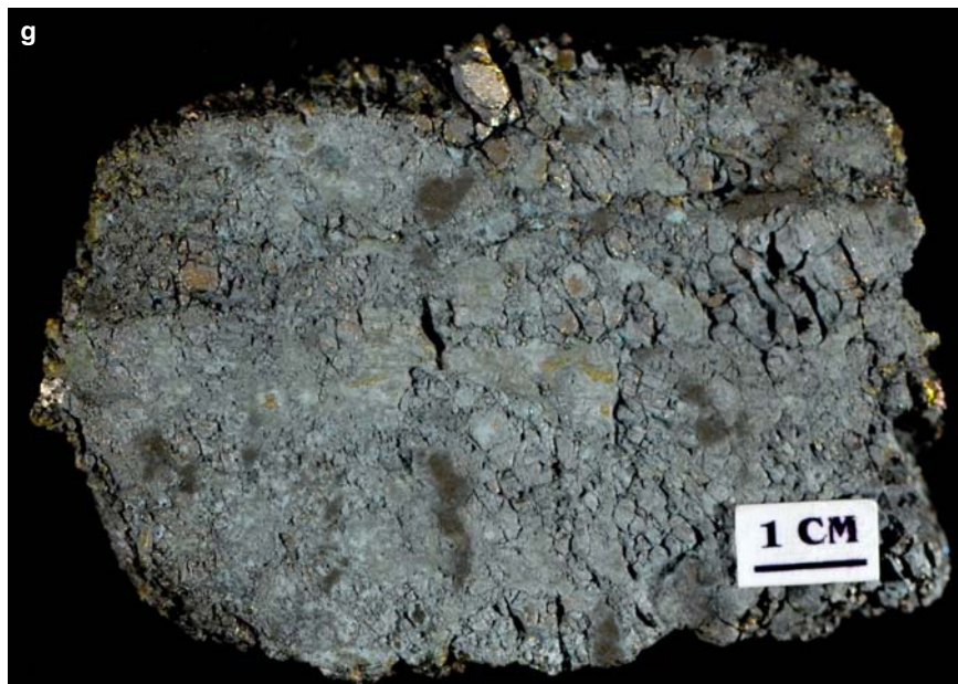
Figure SR2.1g. Creighton mine. Massive chalcopyrite-pentlandite-pyrrhotite. Sample EI-74-309B, collected by Roger Eckstrand from the 126 orebody, 5400 level.
