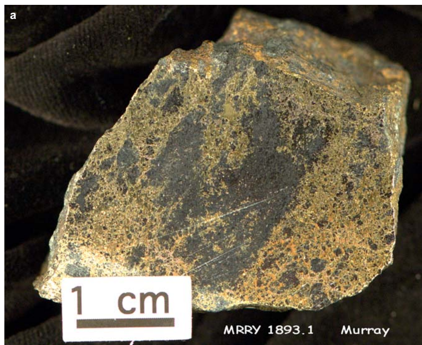
Figure SR1.10a. Murray mine. Semi-massive sulphide chalcopyrite > pyrrhotite, form lace-like texture. Sample MRRY1893-1, collected in 1893 by R. Bell (Walker).
