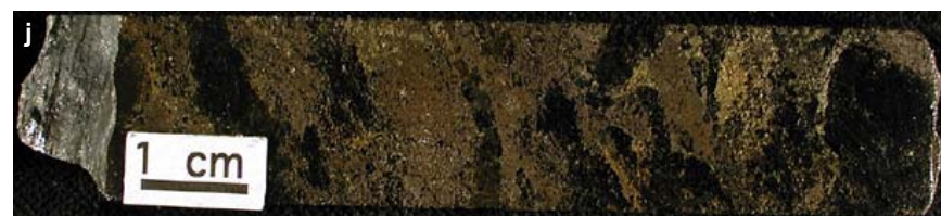
Figure SR1.1j. Blezard deposit. Semi-massive pyrrhotite-pentlandite. Sample 01-AV-234.
