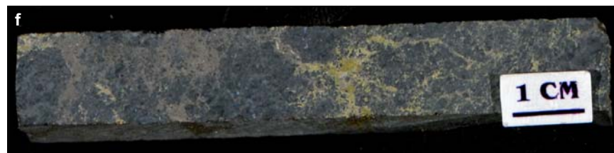
Figure SR3.1f. Copper Cliff deposit. 10% stringer of pyrrhotite-chalcopyrite. Note epidote alteration around stringers. Sample 98-AV-54, bore hole 100505, 257.5-258 ft, 100 orebody.
