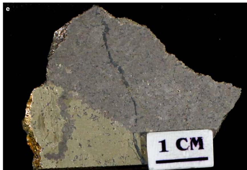
Figure SR1.12e. Victoria Embayment. Massive pyrrhotite-chalcopyrite with minor fine-grained magnetite in the chalcopyrite. Sample 98-AV-85, collected in 1918 by H.V. Ellsworth from Lot 8, Con 2, Denison Township.
