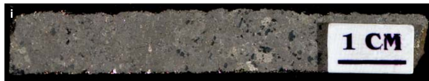
Figure SR3.1i. Copper Cliff deposit. Massive pyrrhotite. Sample 98-AV-57, bore hole 100505, 188.5-189 ft, 100 orebody.
