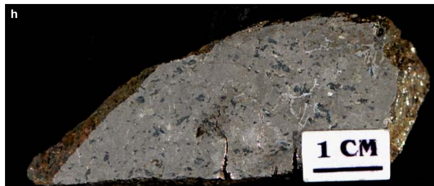
Figure SR1.3h. Crean Hill deposit. Massive marcasite(?) Sample 98-AV-52, 3840 level 3840A.
