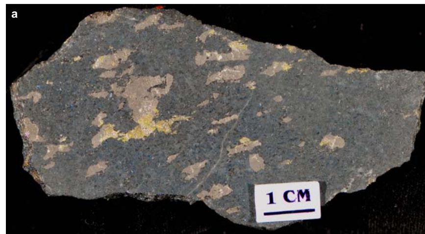
Figure SR4.2a. Frood-Stobie mine. Blebbly to disseminated pyrrhotite-pentlandite with minor chalcopyrite within mafic norite. Sample EI-75-07, collected by Roger Eckstrand from the 2200 level.
