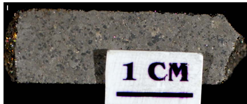
Figure SR3.1l. Copper Cliff deposit. Massive pyrrhotite. Sample 98-AV-60, bore hole 100506, 237.5-238 ft, 100 orebody.
