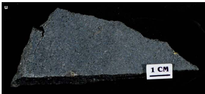
Figure SR1.4u. Creighton mine. 3% blebby and disseminated chalcopyrite-pyrrhotite in sheared, possibly sedimentary, biotite-quartz rock. Sample 02-AV-658, 4030B 5900 Level 4930 drift.
