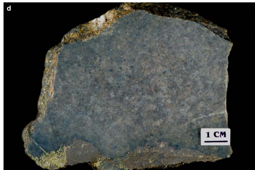
Figure SR1.10d. Murray mine. Massive banded pyrrhotite-chalcopyrite (chalcopyrite veins cross-cutting pyrrhotite) with minor disseminated magnetite. Sample EI-70-04, collected by Roger Eckstrand.
