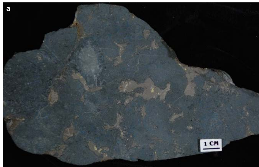
Figure SR1.8a. Little Stobie mine. Blebby to disseminated pyrrhotite with minor chalcopyrite within mafic rock. Sample EI-70-27.
