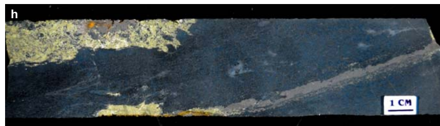
Figure SR1.6h. Kirkwood deposit. Pyrrhotite-chalcopyrite vein and disseminated chalcopyrite-pyrrhotite vein within pelite (2.4 ft @ 3.94% Cu, 0.27% Ni 0.793 oz/ton TPMS). Sample 99-AV-102, collected by Everett Makela from bore hole 93662-1, 2631.6-2634 ft.
