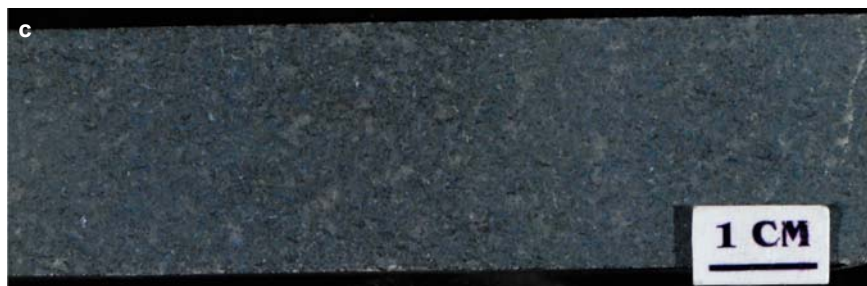
Figure SR2.2c. Segway deposit. Very weakly mineralized quartz diorite with less than 1% sulphide. Note chlorite alteration. Sample 05AV-15, bore hole FNX8001, 217.1 ft.
