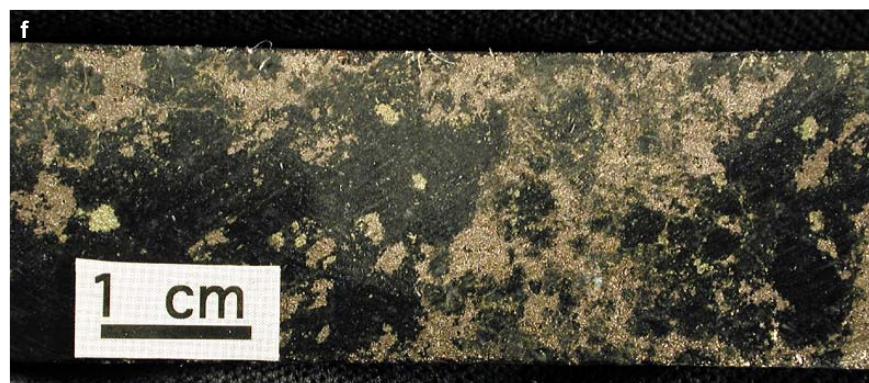
Figure SR3.6f. Totten deposit. 25% blebby pyrrhotite-chalcopyrite. Sample 01-AV-246.
