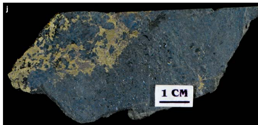
Figure SR1.3j. Crean Hill deposit. 20% blebby chalcopyrite vein and disseminated magnetite. Sample 98-AV-69, collected by Ellsworth from Lot 5, Con 5, Denison Township.
