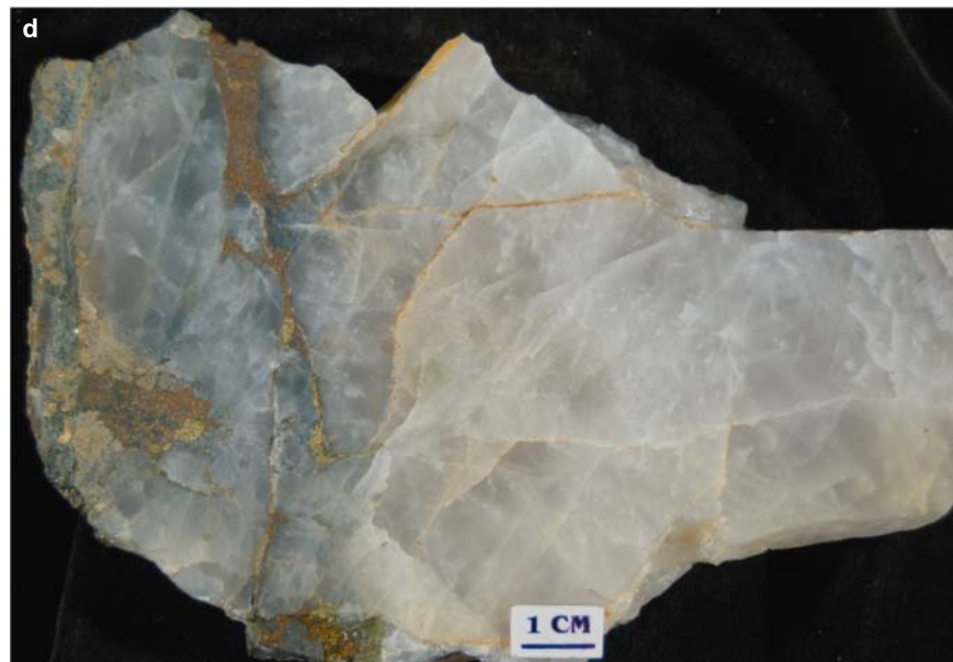
Figure SR4.2d. Frood-Stobie mine. Pyrrhotite-pyrite vein with minor chalcopyrite adjacent to quartz vein. Sample EI-75-11, collected by Roger Eckstrand from the 1200 level.
