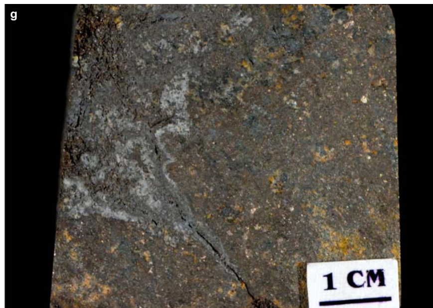
Figure SR1.6g. Kirkwood deposit. Semi-massive pyrrhotite in quartz diorite (barren 0.09% Cu, 0.05% Ni, 0.06 TPM). Sample 99-AV-101, collected by Everett Makela from a surface outcrop.
