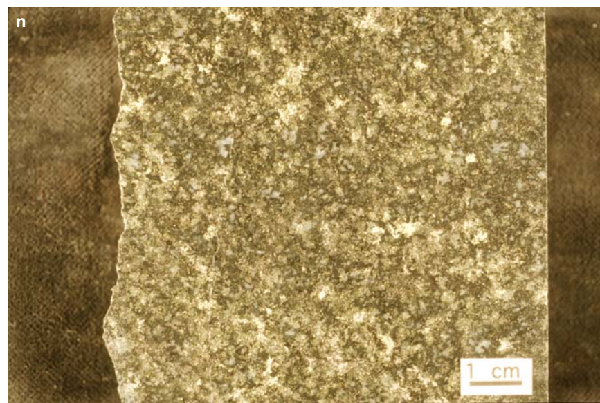
Figure SR1.3n. Crean Hill deposit. Typical ore with 10% blebby chalcopyrite-pyrrhotite-millerite in coarse-grained gabbro. Sample CH-3, Inco collection, collected between approximately 1996 and 1971.
