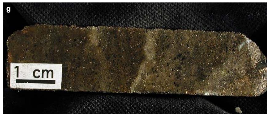
Figure SR1.1g. Blezard deposit. Massive pyrrhotite-pentlandite. Sample 01-AV-230.
