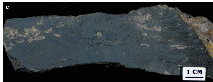
Figure SR1.9c. Mt Nickel deposit. 25% blebby to stinger and disseminated coarse pyrrhotite-chalcopyrite in gabbro. Sample 02-AV-844.
