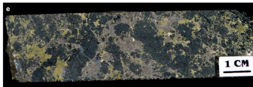
Figure SR3.6e. Totten deposit. Semi-massive interstitial chalcopyrite-pyrrhotite in breccia. Sample 01-AV-245.
