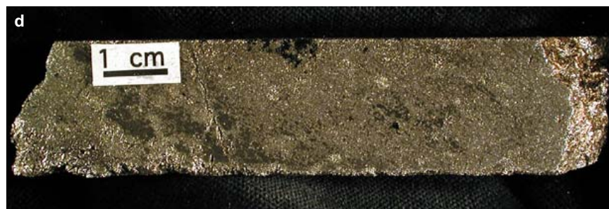
Figure SR3.6d. Totten deposit. Massive pyrrhotite-pentlandite. Sample 01-AV-244.
