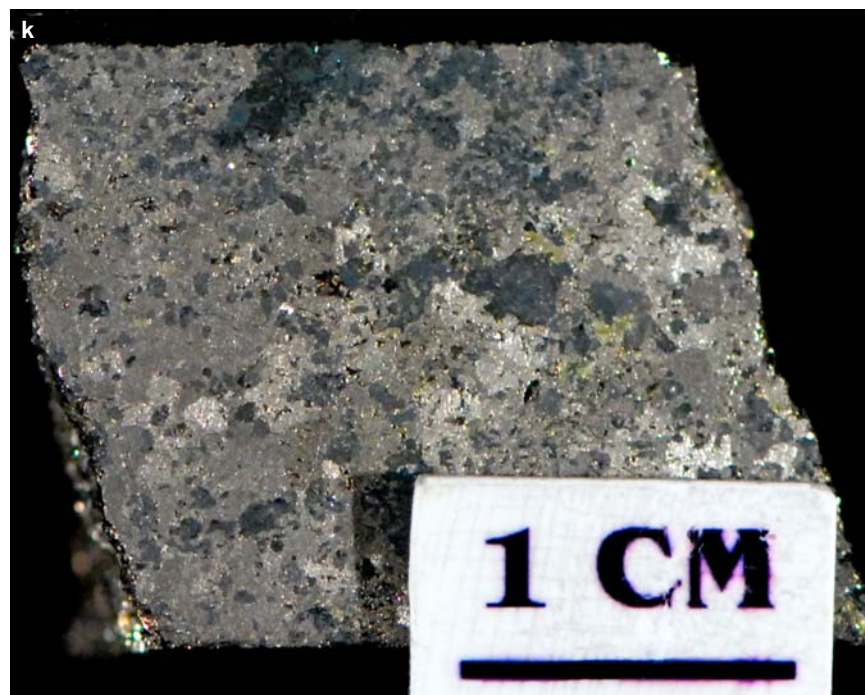
Figure SR3.6k. Totten deposit. Massive pyrrhotite-pentlandite with minor chalcopyrite. Sample 01-AV-251.
