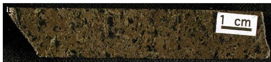
Figure SR1.1i. Blezard deposit. Massive sulphide composed of pyrrhotite-pentlandite. Sample 01-AV-233.
