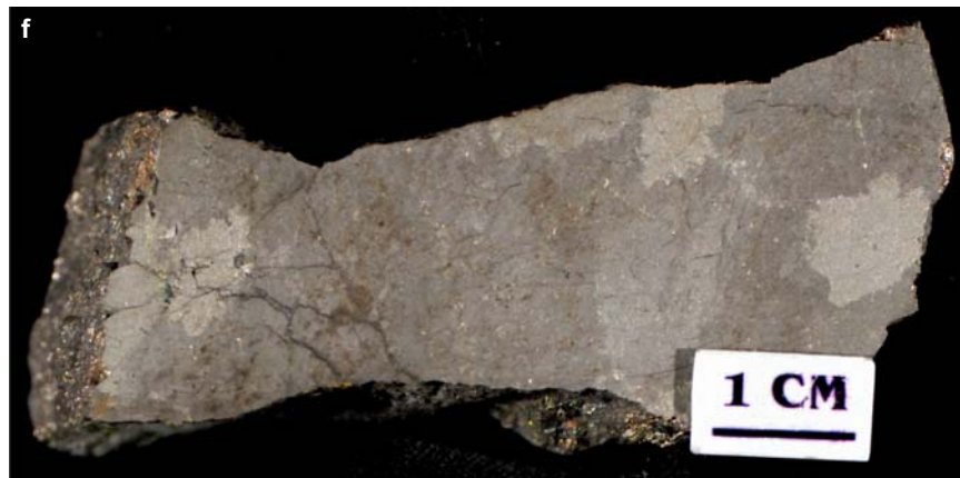
Figure SR3.9f. Worthington mine. Massive pyrrhotite-pentlandite. Note 3 cm pentlandite crystals. Sample 98-AV-65, collected in 1918 by H.V. Ellsworth from Lot 2, Con 2, Drury Township.
