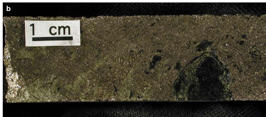
Figure SR3.6b. Totten deposit. Semi-massive chalcopyrite-pyrrhotite in fine-grained amphibolite. Sample 01-AV-242.
