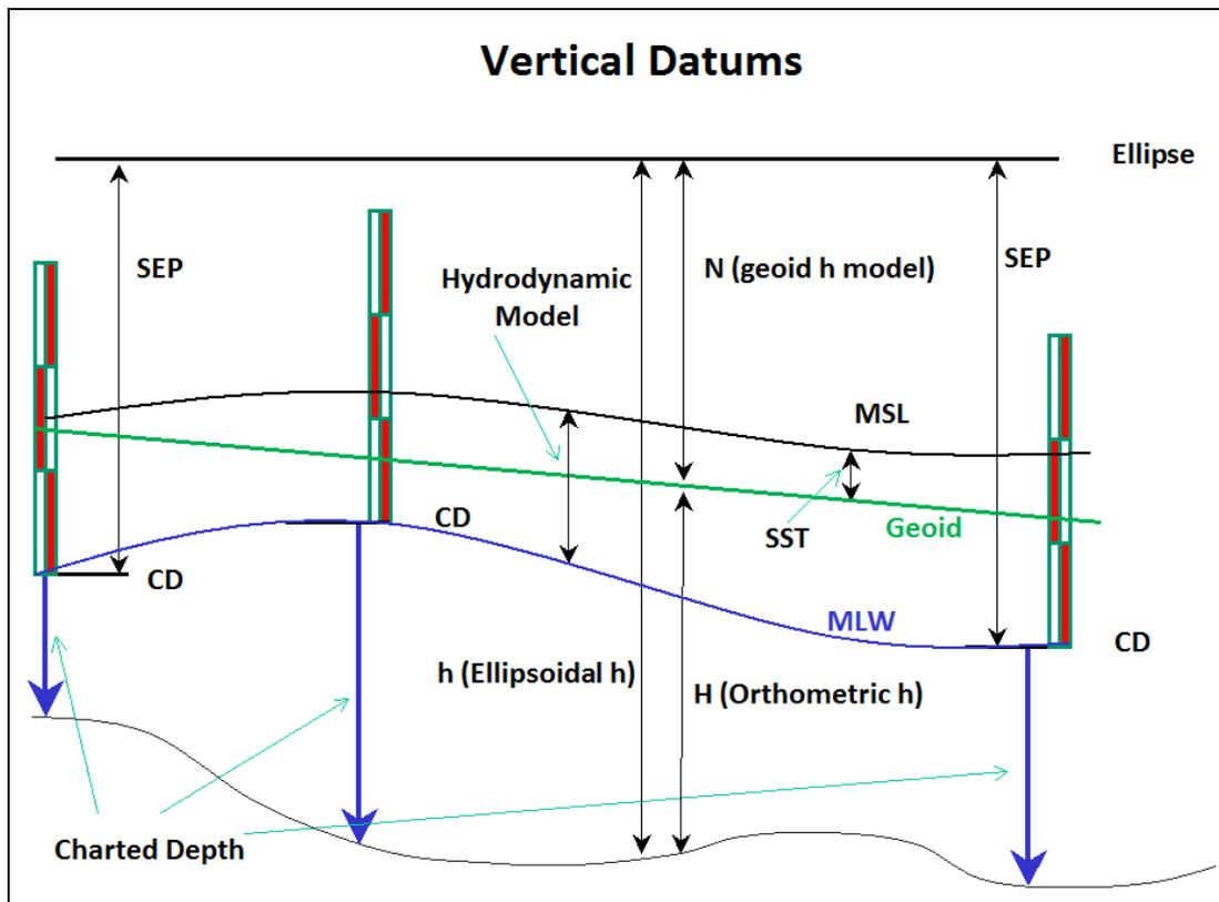
Figure 2: Chart datum, geoid, ellipsoid relationships
