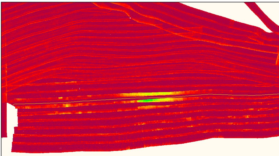
**Figure 8: Sample standard deviation surface with GPS tide error**
