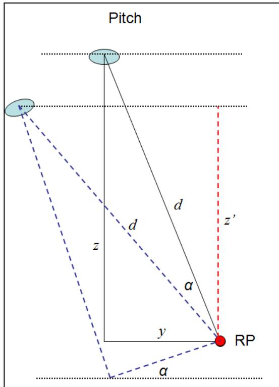
**Figure 5: Effect of vessel pitch on height translation to the vessel reference point**
