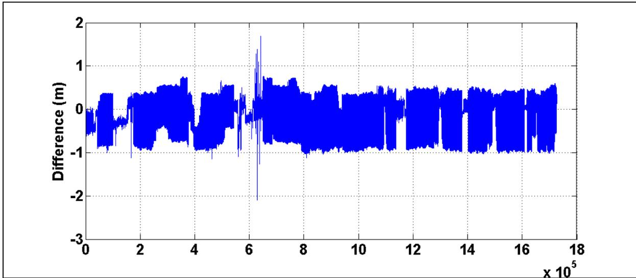
**Figure 14: Plot of difference between GPS Tide and WebTide for section of 2009 survey.
