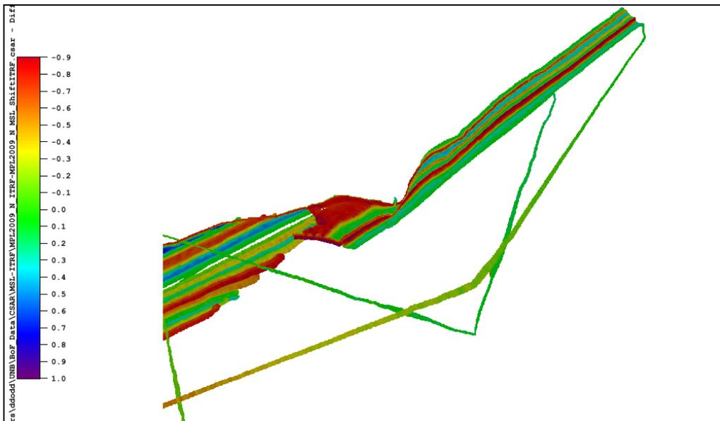
**Figure 13: Difference between GPS Tide and shifted WebTide surfaces. Legend is  $\pm 1$  m**
