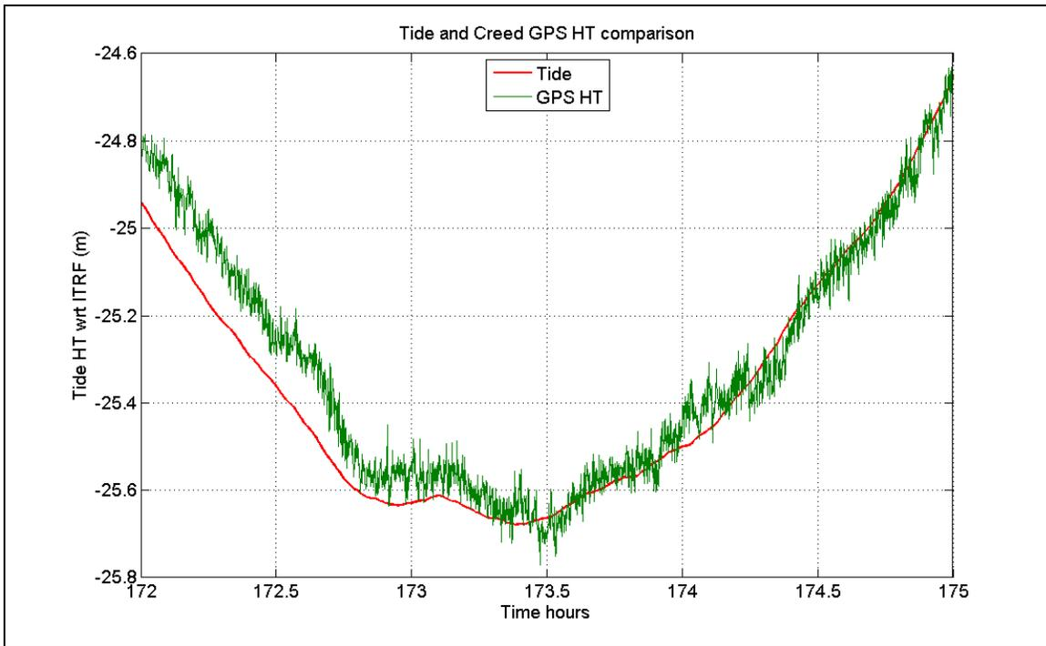
**Figure 7: Creed and Saint John Gauge Comparison. Mean = 0.031 m, standard deviation = 0.074 m ( $1\sigma$ )**
