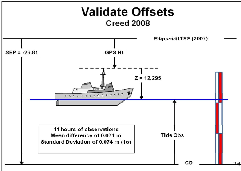
**Figure 6: Creed 2008 Vertical Offset Diagram**
