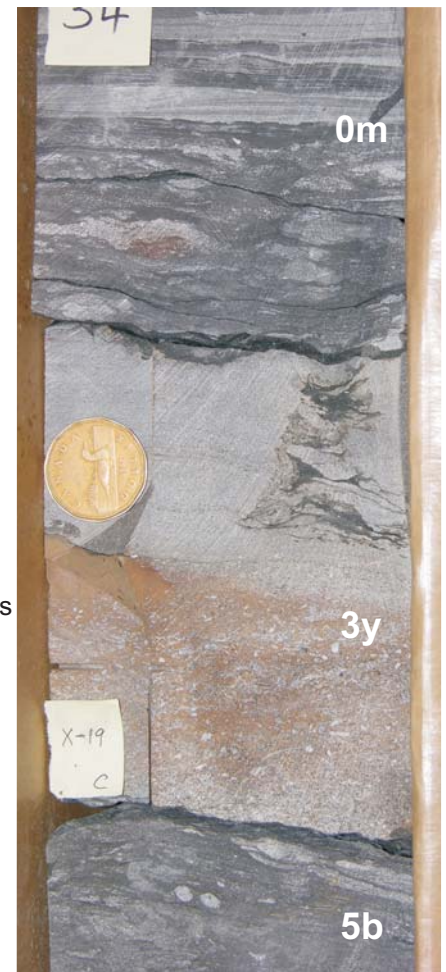
(c) 2401: Facies 0m, mudstone with thin beds of siltstone, some with basal loading. Note thin siltstone bed below laminated sandstone and erosional surface at the top of the sandstone, characteristic of delta-front turbidites.
