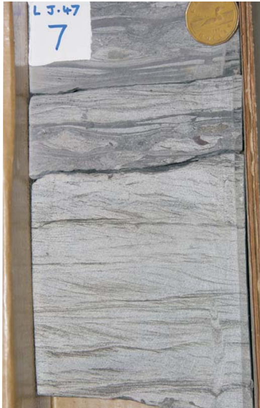
(c) 2355: Facies 5s, tidal flat sandstone overlain by facies 5 m, tidal flat sandstone and mudstone.
