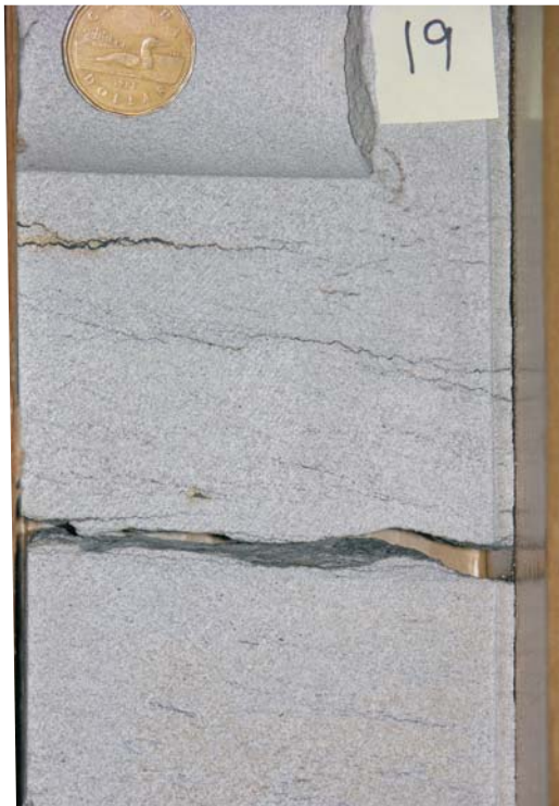
(a) 2393: Medium sandstone of facies 4o. Note cross bedding picked out by thin mud drapes, and the presence of Ophiomorpha burrows.
