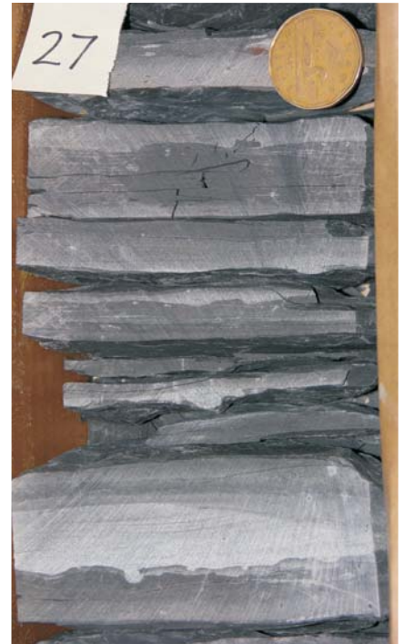
(c) 2401: Facies 0m, mudstone with thin beds of siltstone, some with basal loading. Note thin siltstone bed below laminated sandstone and erosional surface at the top of the sandstone, characteristic of delta-front turbidites.
