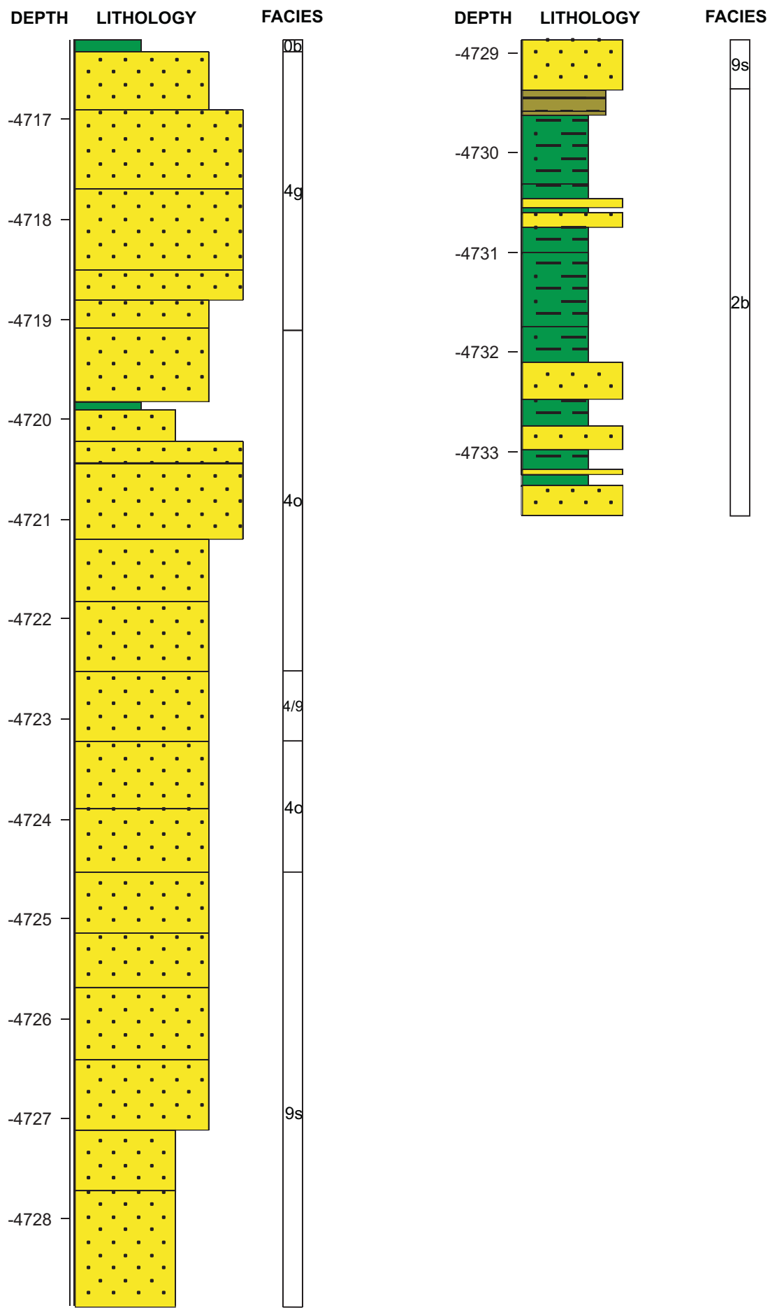
Figure 17 (con't): Summary log of core 3 from the Venture B-13 well. Lithofacies have been reinterpreted from Karim et al., 2010.
