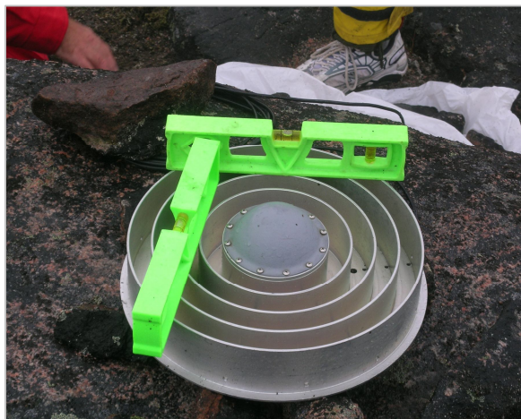
Installation of the high precision choke ring GPS antenna.
