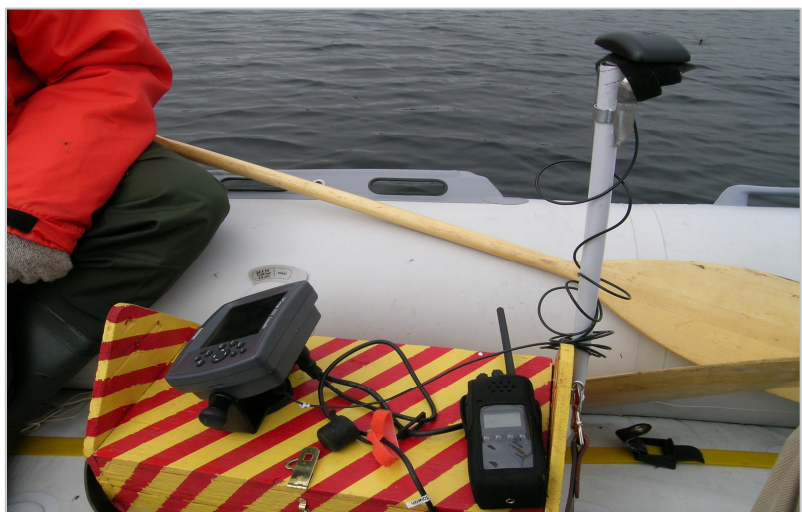
Equipment used for collecting bathymetric data: sonar fish finder and GPS receiver.
