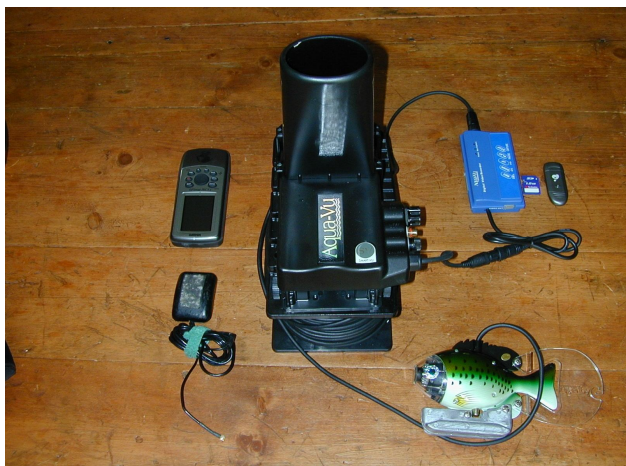
Underwater video camera equipment used to observe T-Lake intake pipes.
