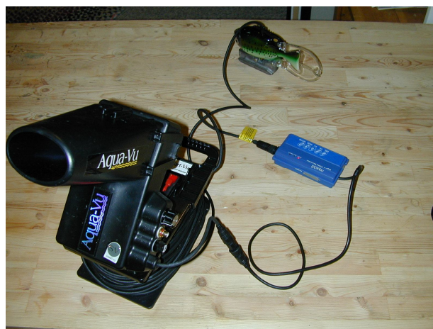
Underwater video camera equipment used to observe T-Lake intake pipes.
