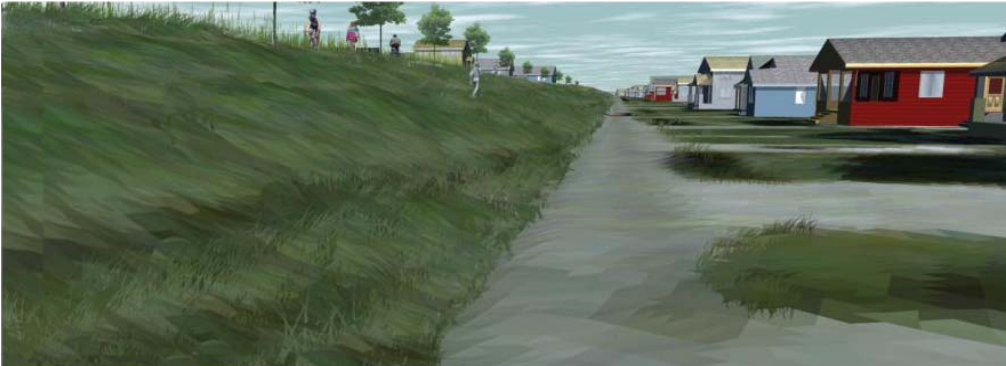
B) Image: Visualization of raised dike (to protect against climate change-induced sea level rise over the next century). In this case the additional space required to raise the dike has impacted an existing roadway. Image credit: David Flanders, UBC-CALP
