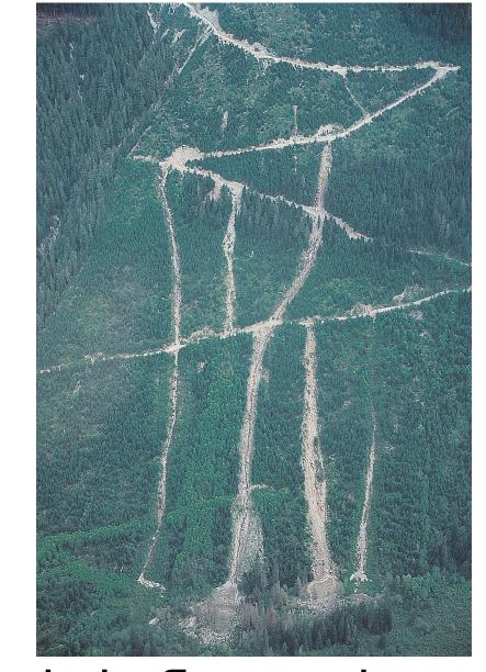
Debris flows triggered where the logging road concentrated runoff.
