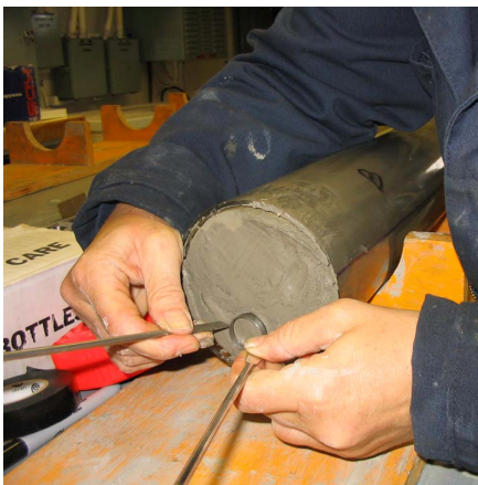
Figure 6.3 Inserting the constant volume sampler.
