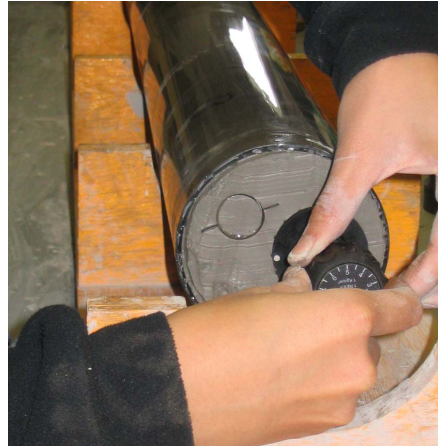
Figure 6.2 Taking a Torvane measurement.
