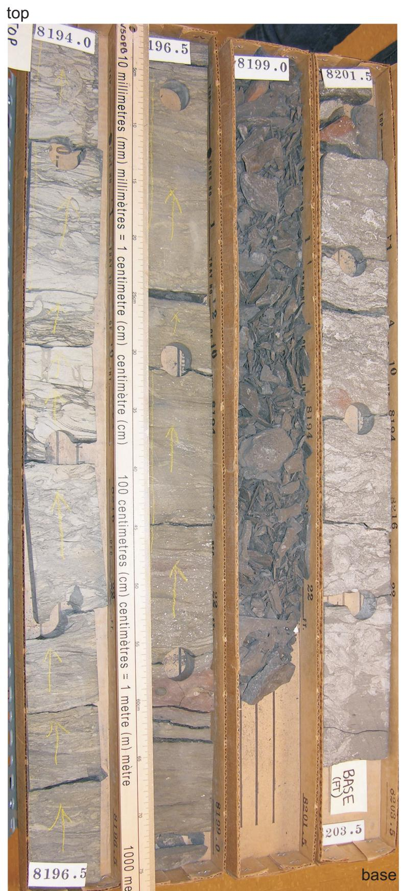
Figure 8: Core photographs of core 1, Mic Mac D-89, Middle Member, Missisauga Formation, 2497.53-2500.43 m.
