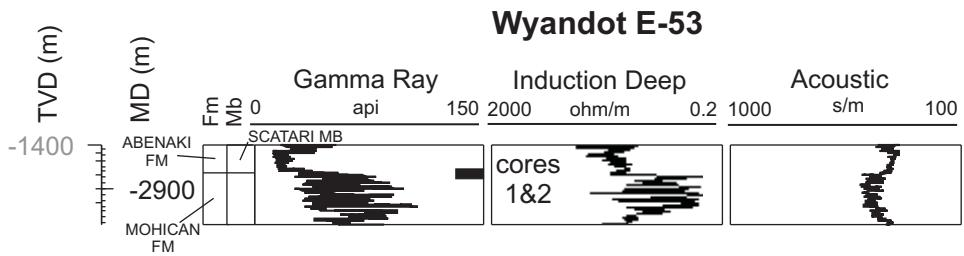
Figure 42: Summary logs of the Wyandot E-53 wells (MD = measured depth, TVD = true vertical depth). Formation and member picks from MacLean and Wade (1993). Core 2 was used in this study.
