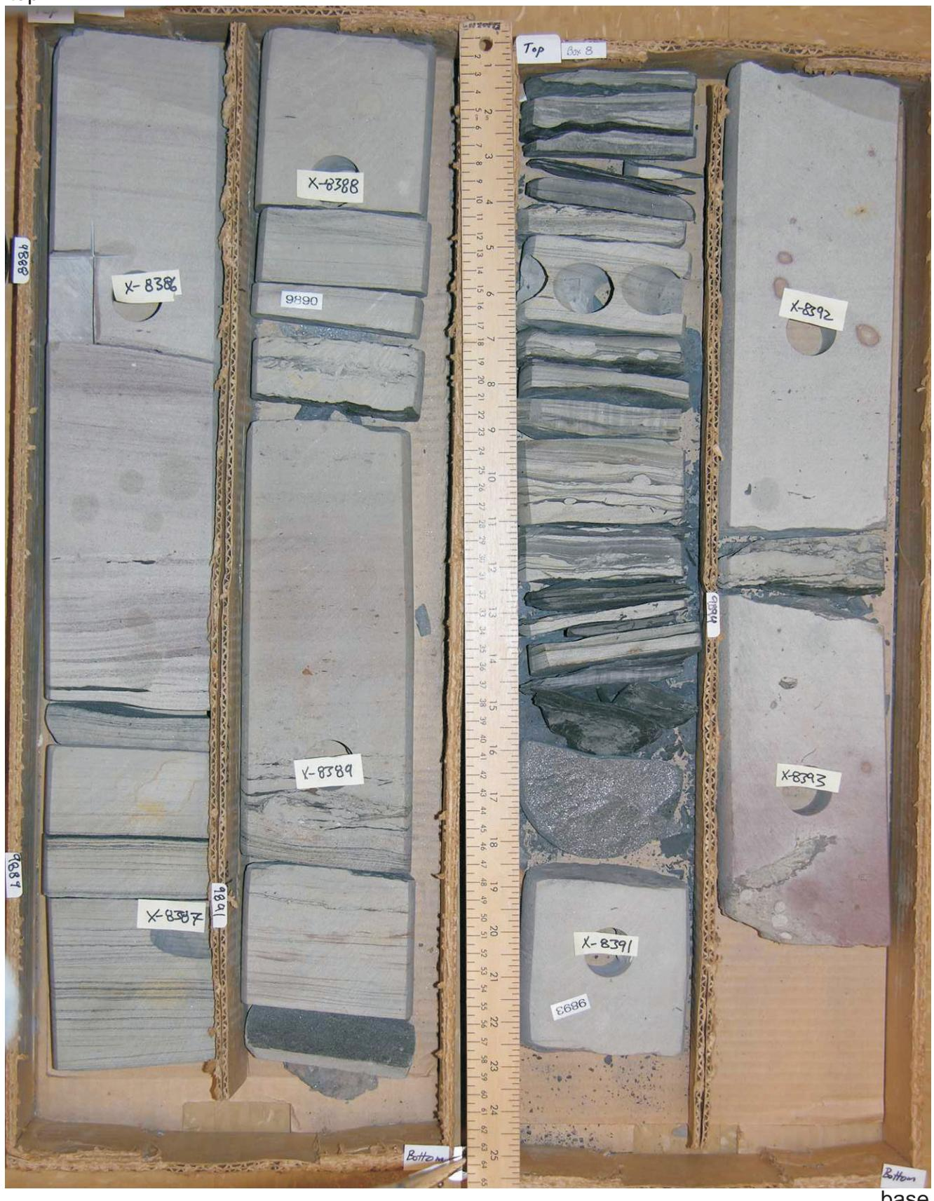
Figure 4 (con't): Core photographs of core 1, Marmora P-35, Upper Member, Missisauga Formation, 3013.75 - 3015.90 m.
