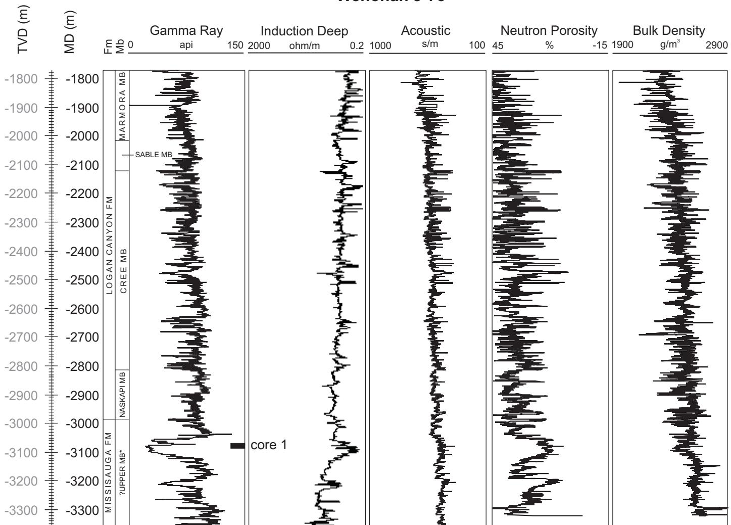
Figure 30: Summary logs of the Wenonah J-75 well (MD = measured depth, TVD = true vertical depth). Formation and member picks from MacLean and Wade (1993). \* = source from BASIN Database (<http://basin.gdr.nrcan.gc.ca/>), where no reference is given.
