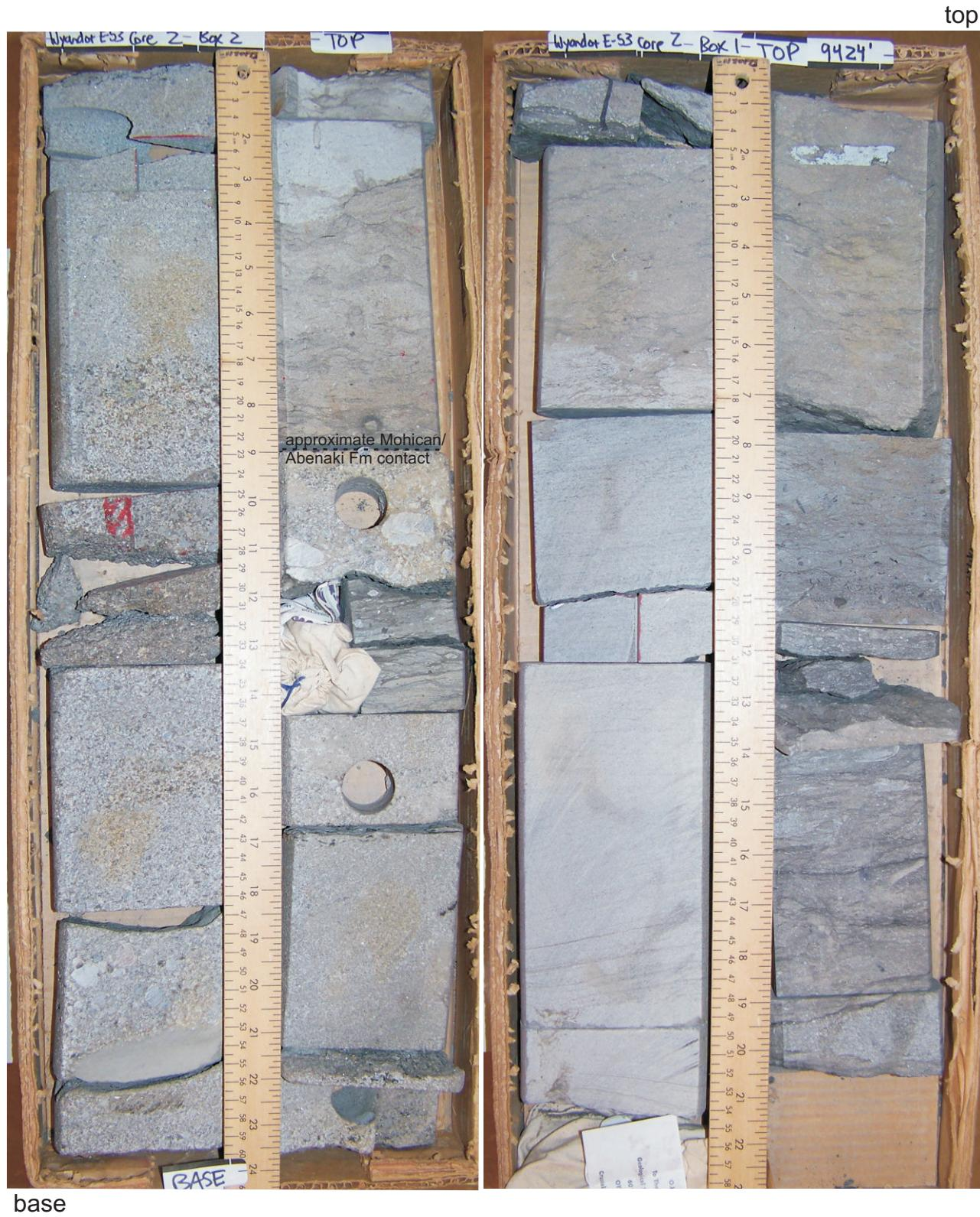
Figure 44: Photographs of core 2 from the Wyandot E-53 well, across the contact between the Mohican Formation and Scatarie Member of the Abenaki Formation 2872.45-2874.57 m.
