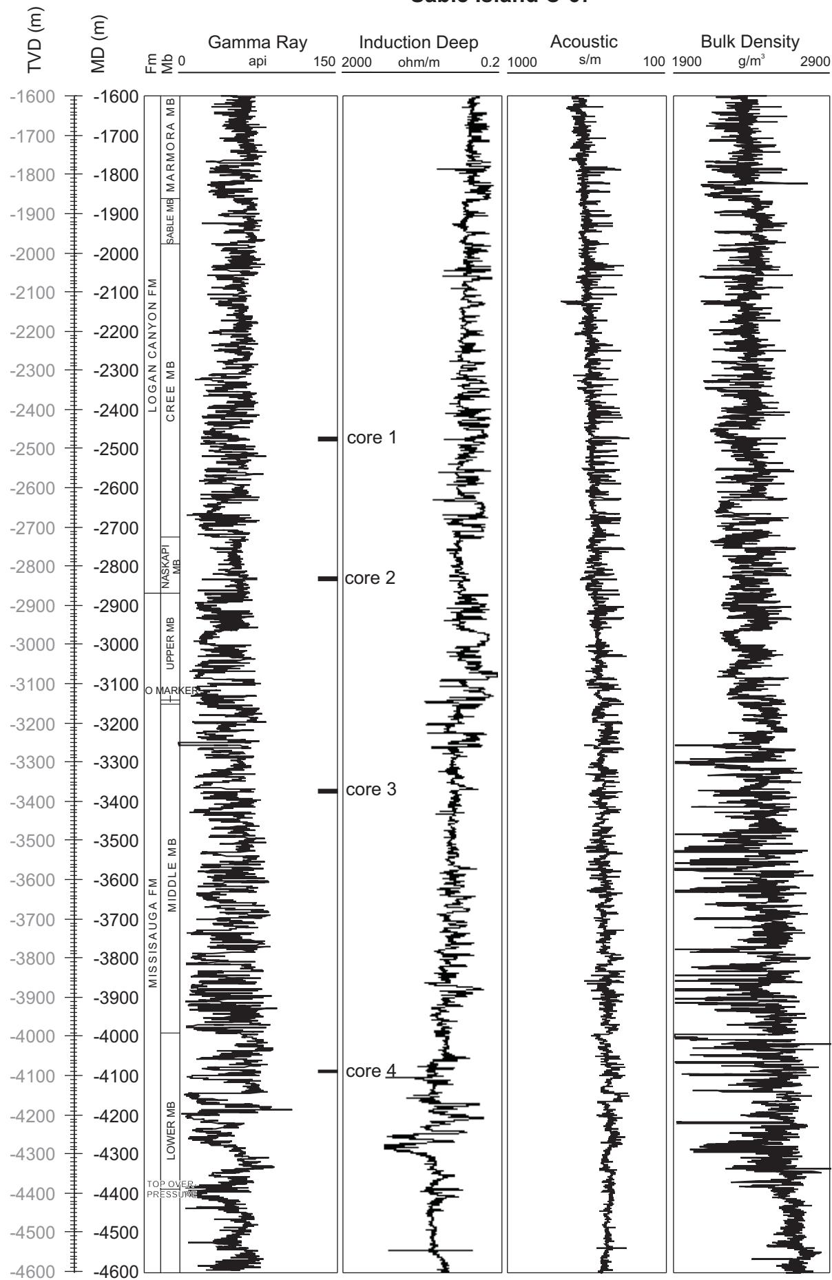
Figure 22: Summary logs of the Sable Island C-67 well (MD = measured depth, TVD = true vertical depth). Formation and member picks from MacLean and Wade (1993).
