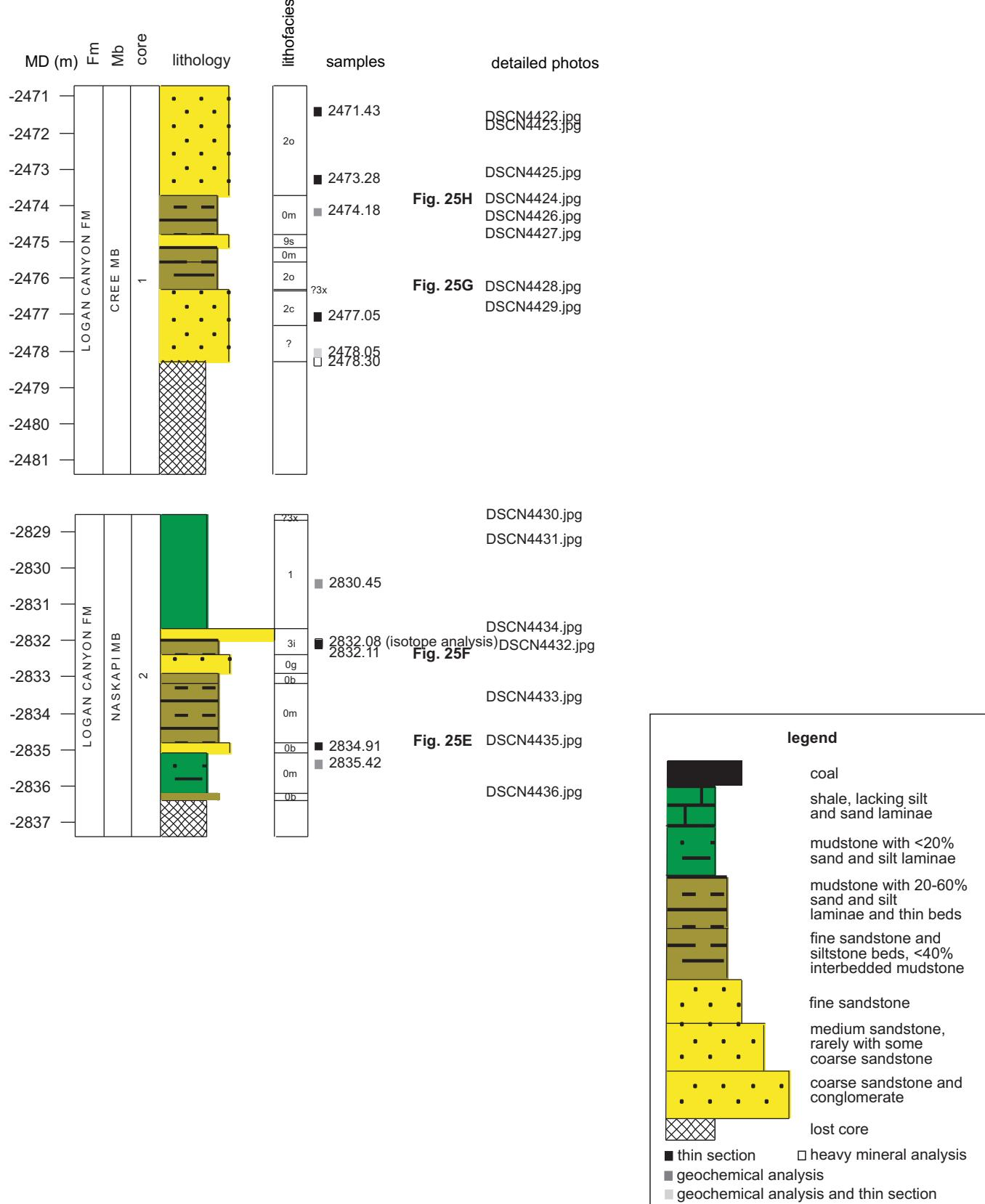
Figure 23: Summary log of conventional core 1-2 from the Sable Island C-67 well (MD = measured depth). Lithofacies are defined in Table 1. Formation and member picks from MacLean and Wade (1993).
