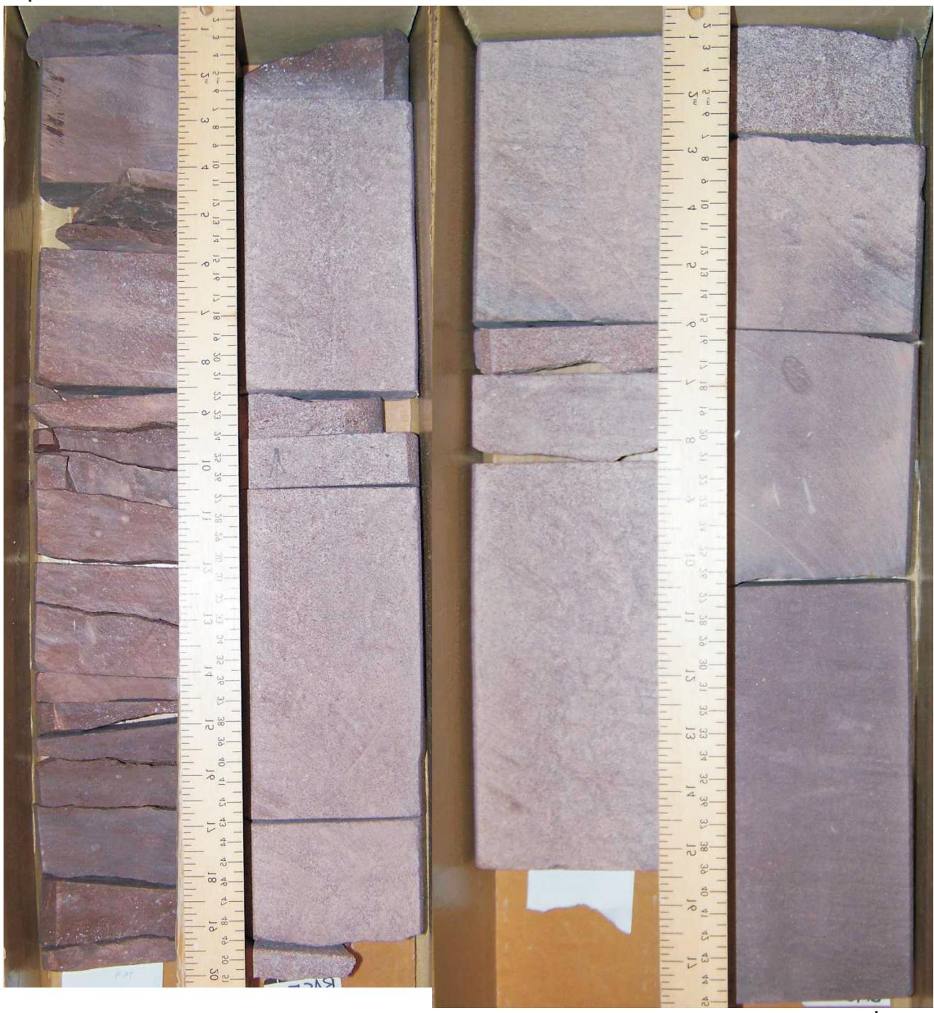
Figure 36: Core photographs of core 1, Mic Mac H-86, Mohican Formation, 4717.70 - 4719.43 m.
