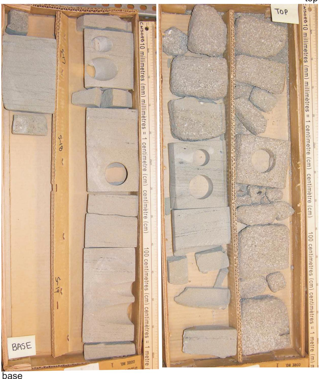
Figure 12 (con't): Core photographs of core 1, Mic Mac J-77, Middle Member, Missisauga Formation, 2813.96-2818.02m.
