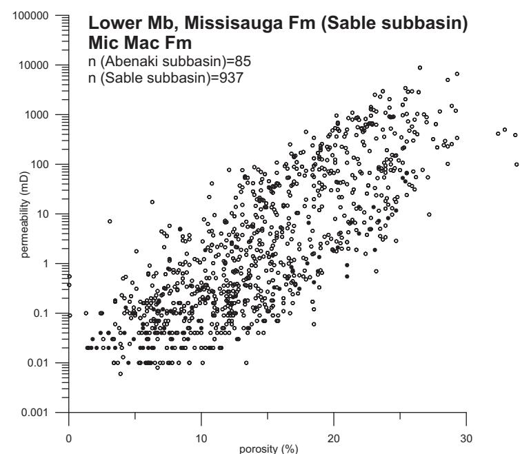
Figure 46: Compiled porosity and permeability measurements by subbasin and stratigraphic unit. Values were taken from small plugs samples in conventional core, made by the operating company.
