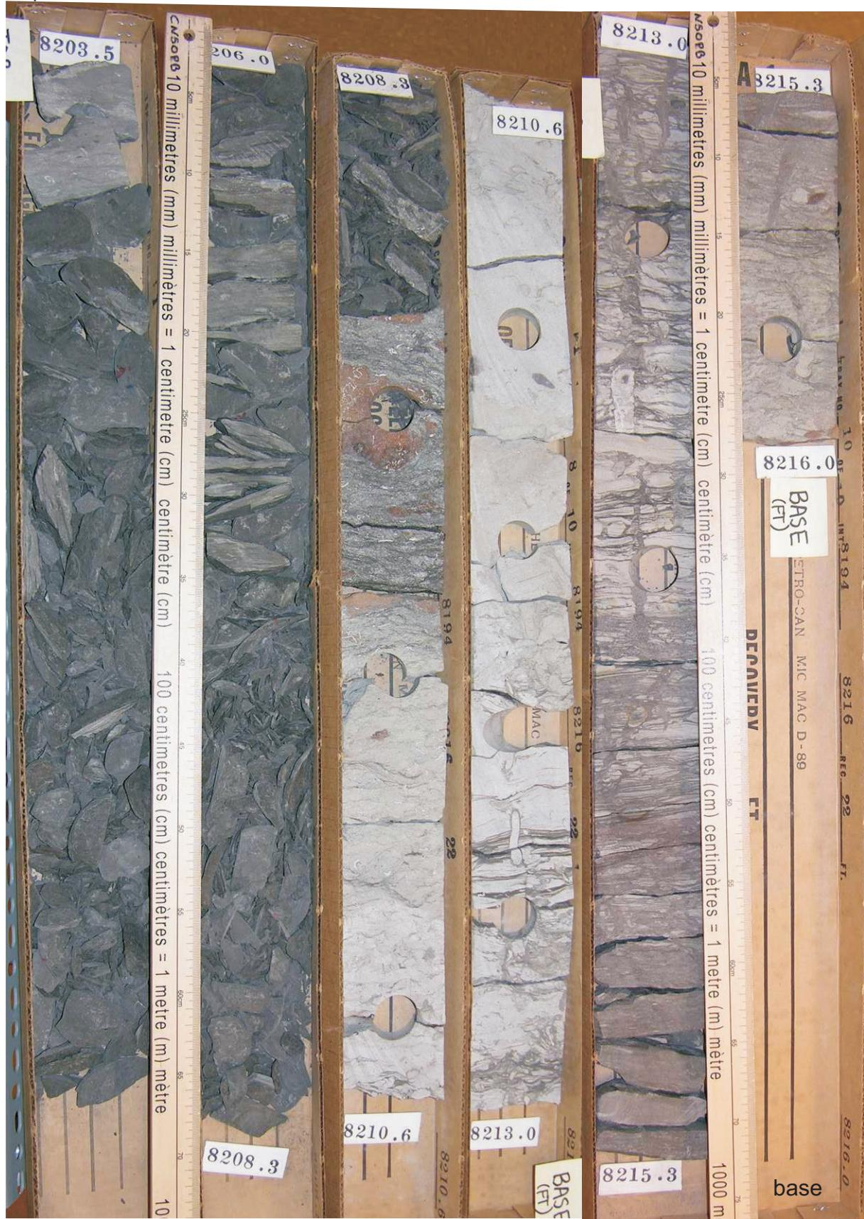
Figure 8 (con't): Core photographs of core 1, Mic Mac D-89, Middle Member, Missisauga Formation, 2500.43-2504.24 m.
