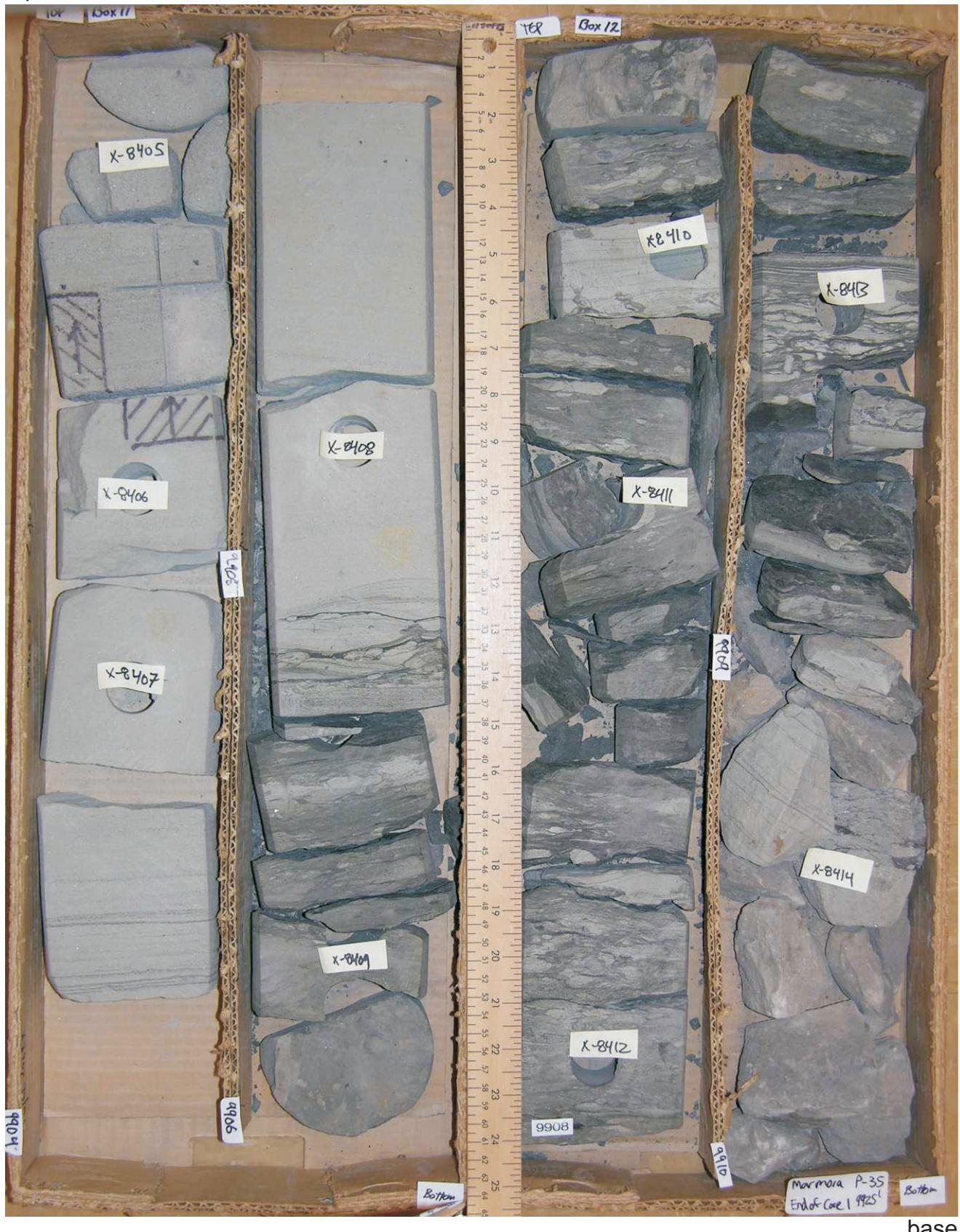
Figure 4 (con't): Core photographs of core 1, Marmora P-35, Upper Member, Missisauga Formation, 3018.15 - 3020.55 m.
