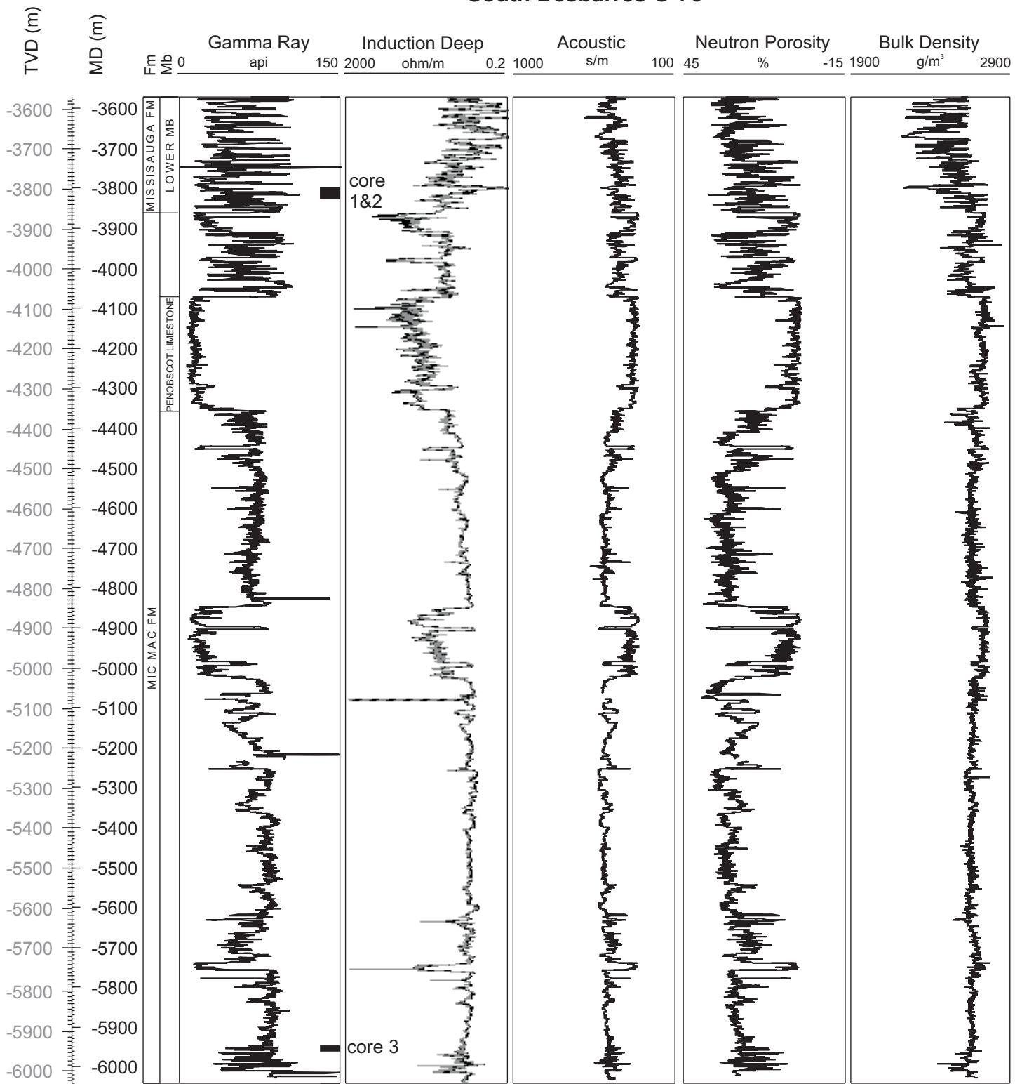
Figure 26: Summary logs of the South Desbarres O-76 well (MD = measured depth, TVD = true vertical depth). Formation and member picks from MacLean and Wade (1993).
