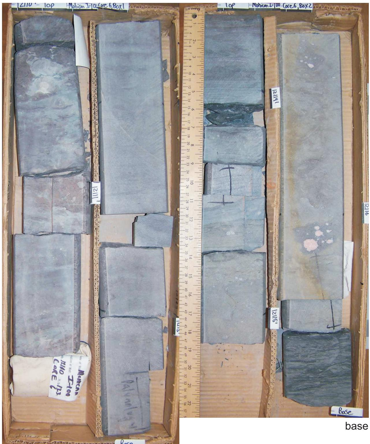
Figure 40: Photographs of core 6 in the Mohican I-100 well, from the Mohican Formation, 3691.13-3693.16 m.
