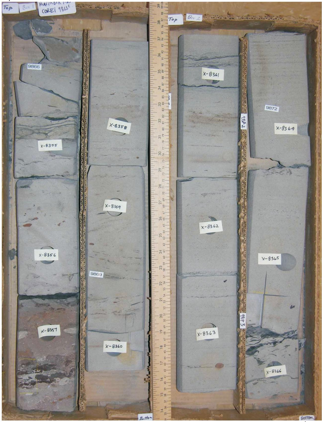
Figure 4: Core photographs of core 1, Marmora P-35, Upper Member, Missisauga Formation, 3007.15 - 3009.45 m.
