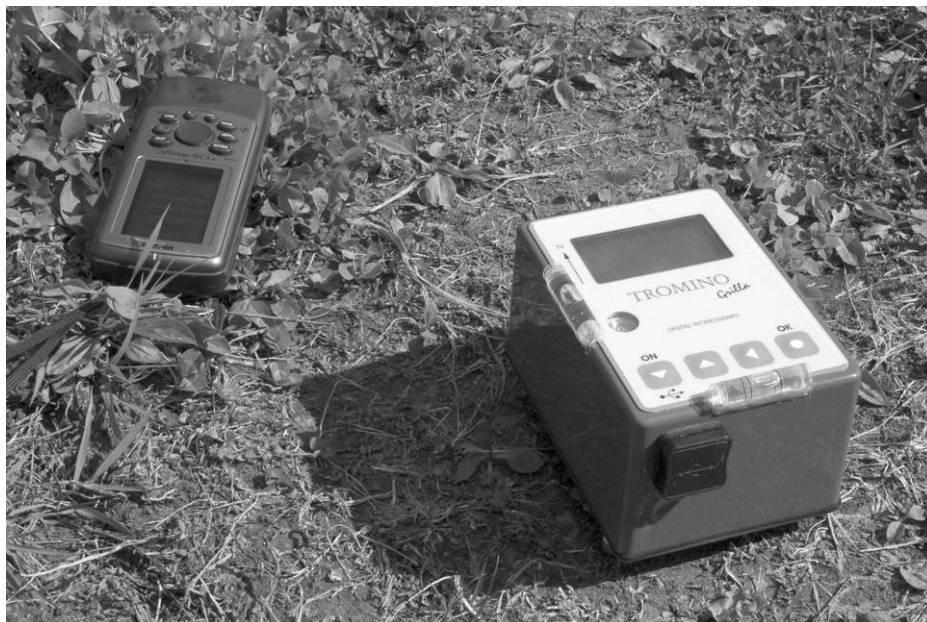
Figure 2-12. Tromino three-component noise monitoring seismograph (on right).
