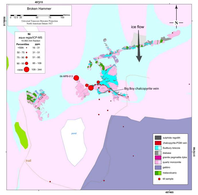
**Map 5.** Abundance of nickel in the <0.063 mm fraction of till proximal to the Broken Hammer occurrence (detailed bedrock geology from Peterson et al., 2004; regional bedrock geology from Ames et al., 2005) (Datum NAD27).
