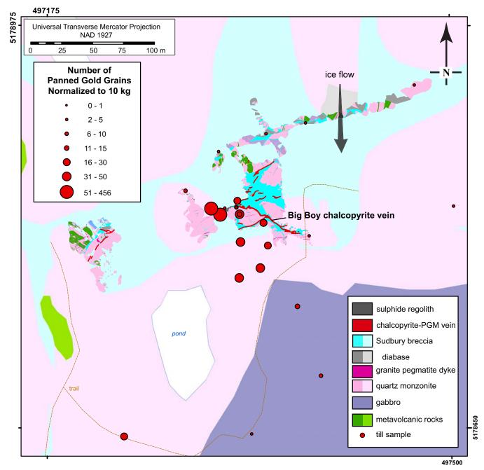
**Map 15.** Abundance of gold grains in till (normalized to a 10 kg sample weight) proximal to the Broken Hammer site (detailed bedrock geology from Peterson et al. 2004; regional bedrock geology from Ames et al., 2005) (Datum NAD27).
