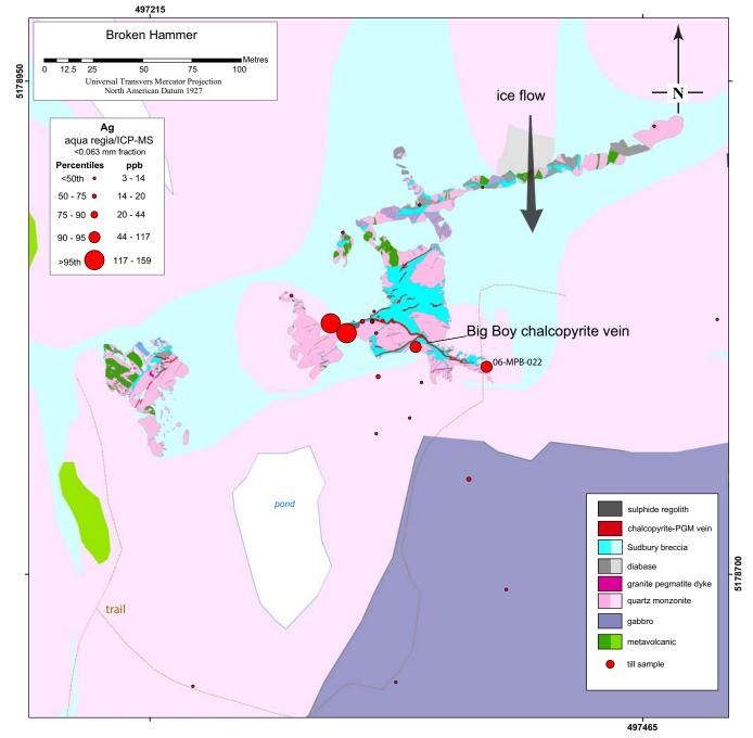
**Map 6.** Abundance of silver in the <0.063 mm fraction of till proximal to the Broken Hammer occurrence (detailed bedrock geology from Peterson et al., 2004; regional bedrock geology from Ames et al., 2005) (Datum NAD27).
