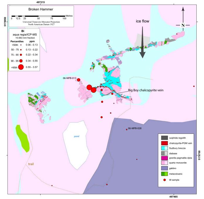
**Map 7.** Abundance of bismuth in the <0.063 mm fraction of till proximal to the Broken Hammer occurrence (detailed bedrock geology from Peterson et al., 2004; regional bedrock geology from Ames et al., 2005) (Datum NAD27).
