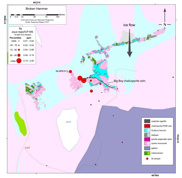
**Map 10.** Abundance of tellurium in the <0.063 mm fraction of till proximal to the Broken Hammer occurrence (detailed bedrock geology from Peterson et al., 2004; regional bedrock geology from Ames et al., 2005) (Datum NAD27).
