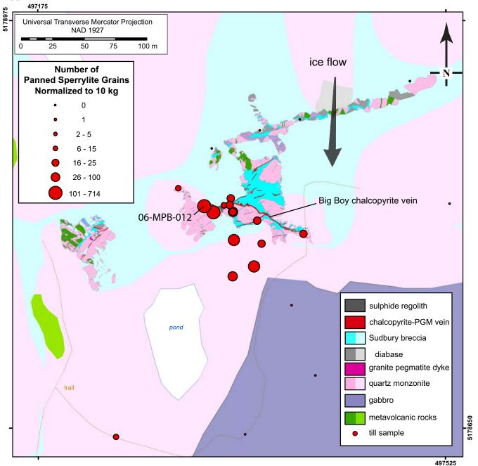
**Map 16.** Abundance of sperrylite grains in till (normalized to a 10 kg sample weight) proximal to the Broken Hammer site (detailed bedrock geology from Peterson et al. 2004; regional bedrock geology from Ames et al., 2005) (Datum NAD27).
