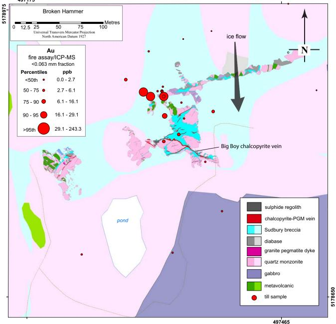
**Map 3.** Abundance of gold in the <0.063 mm fraction of till proximal to the Broken Hammer occurrence (detailed bedrock geology from Peterson et al., 2004; regional bedrock geology from Ames et al., 2005) (Datum NAD27).
