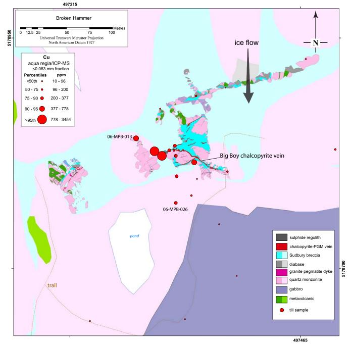
**Map 4.** Abundance of copper in the <0.063 mm fraction of till proximal to the Broken Hammer occurrence (detailed bedrock geology from Peterson et al., 2004; regional bedrock geology from Ames et al., 2005) (Datum NAD27).
