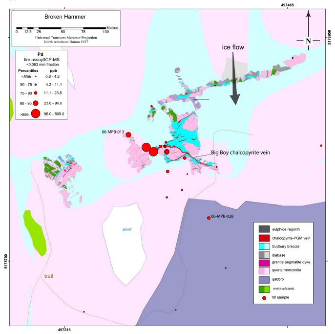
**Map 2.** Abundance of palladium in the <0.063 mm fraction of till proximal to the Broken Hammer occurrence (detailed bedrock geology from Peterson et al., 2004; regional bedrock geology from Ames et al., 2005) (Datum NAD27).
