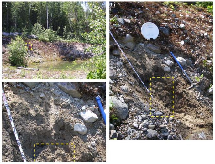
Till sample site 06-MPB-038 in a borrow pit, 1500 m south of the Broken Hammer occurrence: a) overview of the sample site in the south wall of a pit; b and c) close-up of sandy till that was sampled. Sample site is indicated by a yellow dashed line.
