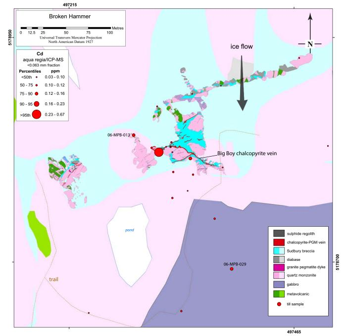
**Map 8.** Abundance of cadmium in the <0.063 mm fraction of till proximal to the Broken Hammer occurrence (detailed bedrock geology from Peterson et al., 2004; regional bedrock geology from Ames et al., 2005) (Datum NAD27).
