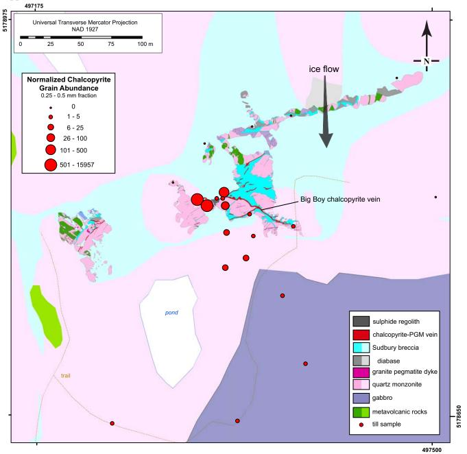
**Map 17.** Abundance of chalcopyrite grains in till (normalized to a 10 kg sample weight) proximal to the Broken Hammer site (detailed bedrock geology from Peterson et al. 2004; regional bedrock geology from Ames et al., 2005) (Datum NAD27).
