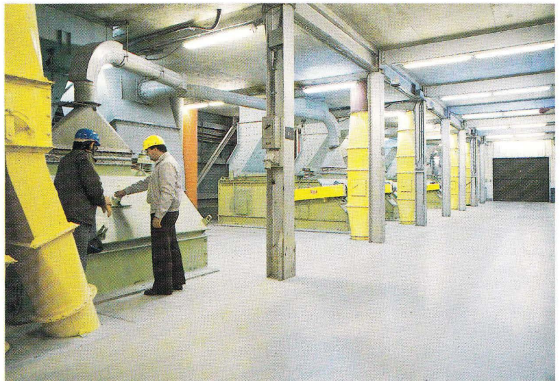
Asbestos fibre processing through fully enclosed equipment.
