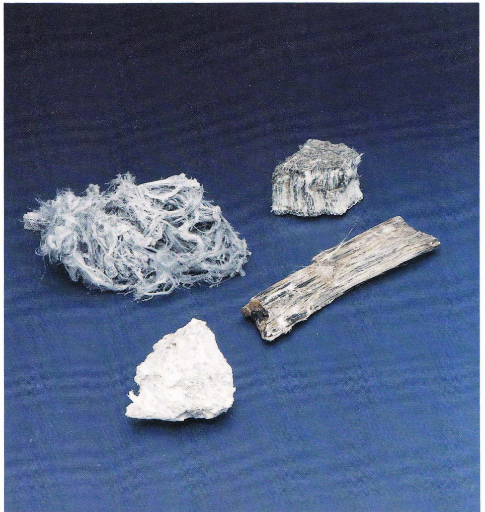
Three types of asbestos fibre have commercial value: amosite (bottom left), crocidolite (top left), and chrysotile (top and bottom right). Chrysotile accounts for 95 percent of the commercial use of asbestos.
