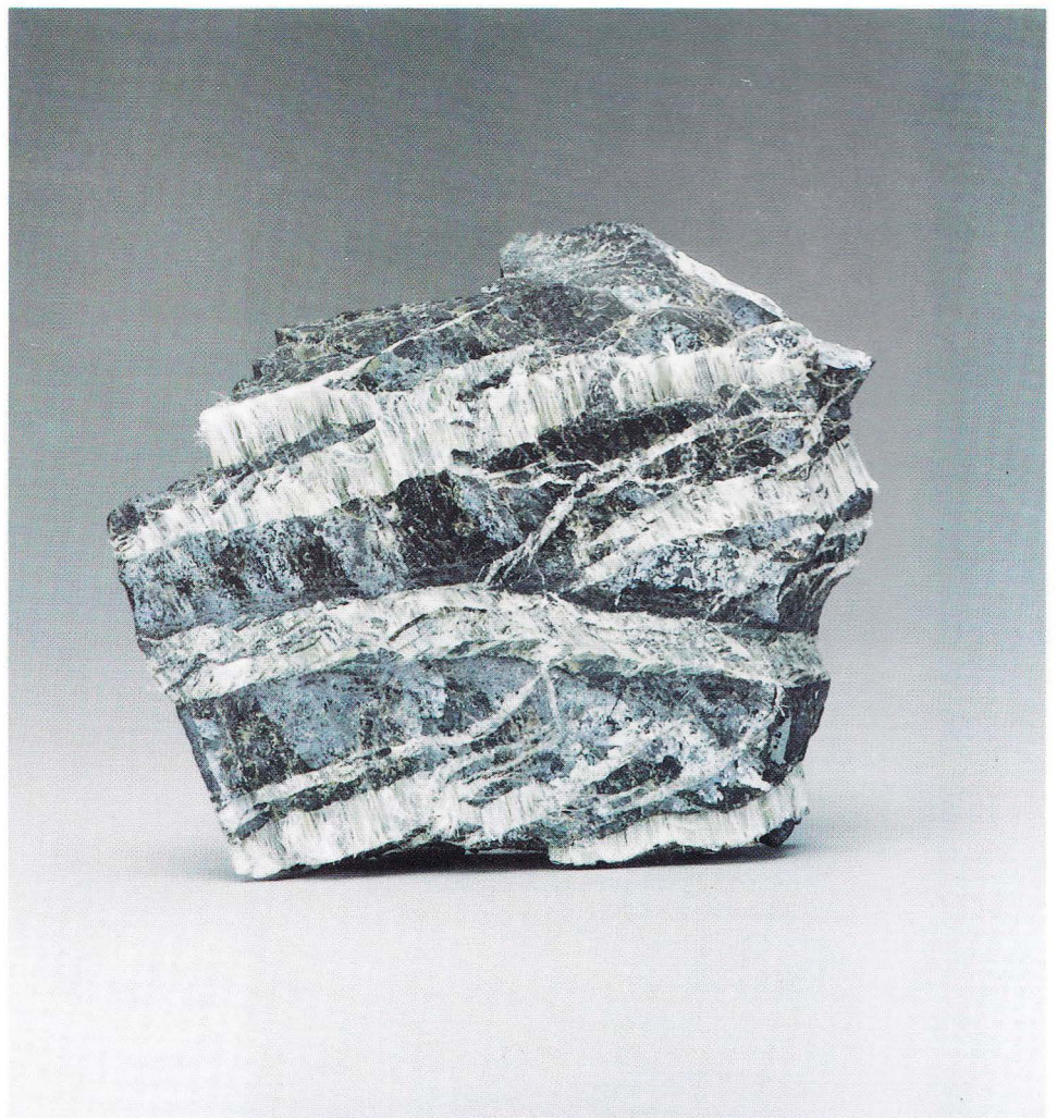
Chrysotile asbestos is found in cross fibre veins zigzagging through the host rock.
