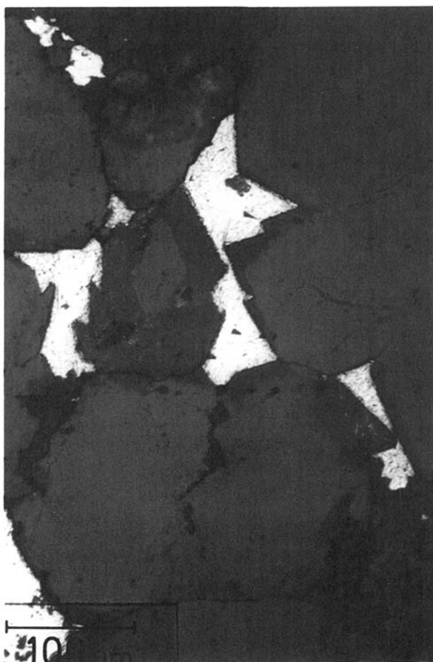
Figure 8.2-2. Photomicrograph illustrating detrital quartz grains (light grey) partially surrounded by silica overgrowths (dark grey) in characteristic straight-edge contact with galena cement (white), Yava (from Sangster and Vaillancourt, 1990b). GSC 204077-F
