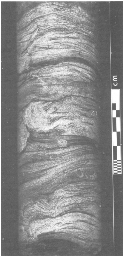
Figure 38. Distorted sandstone and siltstone laminations. Note small, horizontal, sand-filled burrow and dark grey mudstone flasers in sandstone laminations. Fording River (Sec. 75-24), Mist Mountain Formation.
