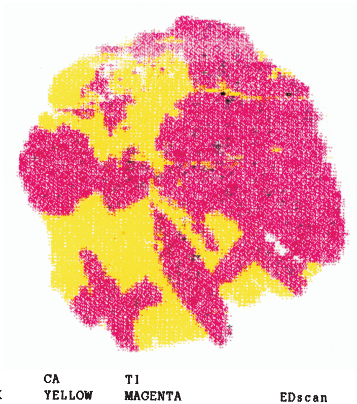
Plate 4. X-ray scan of Plate 3 (300x) illustrating distribution of Nb minerals (black) Ti minerals, rutile (red) and of Ca minerals-dolomite (yellow).
