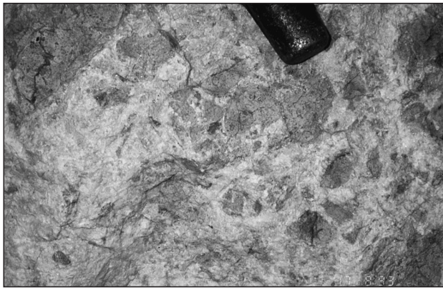
Figure 72. Quartz breccia vein; Mount Skukum deposit, Yukon Territory. Scale object is the blunt end of a geological hammer (photograph by K.H. Poulsen). GSC 1999-016K
