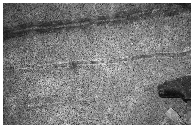
Figure 82. Sheeted quartz veins in granodiorite; Eagle zone, Dublin Gulch deposit, Yukon Territory (photograph by K.H. Poulsen). GSC 1999-0160
