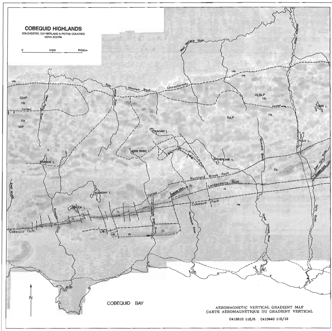
Figure 3. Black and white reproduction of aeromagnetic vertical gradient map from 1:50 000 colour original print. Superimposed simplified geological data locating structural and lithological features discussed in this report.
