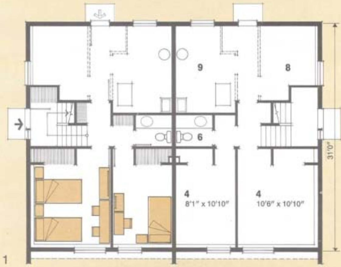
In this composite design two different two-storey houses are brought together. The house on the left is a two-bedroom house (floor area 895 sq. ft.) and the house on the right is design 1.07 (floor area 1068 sq. ft.) which is illustrated in Part one of this book.
