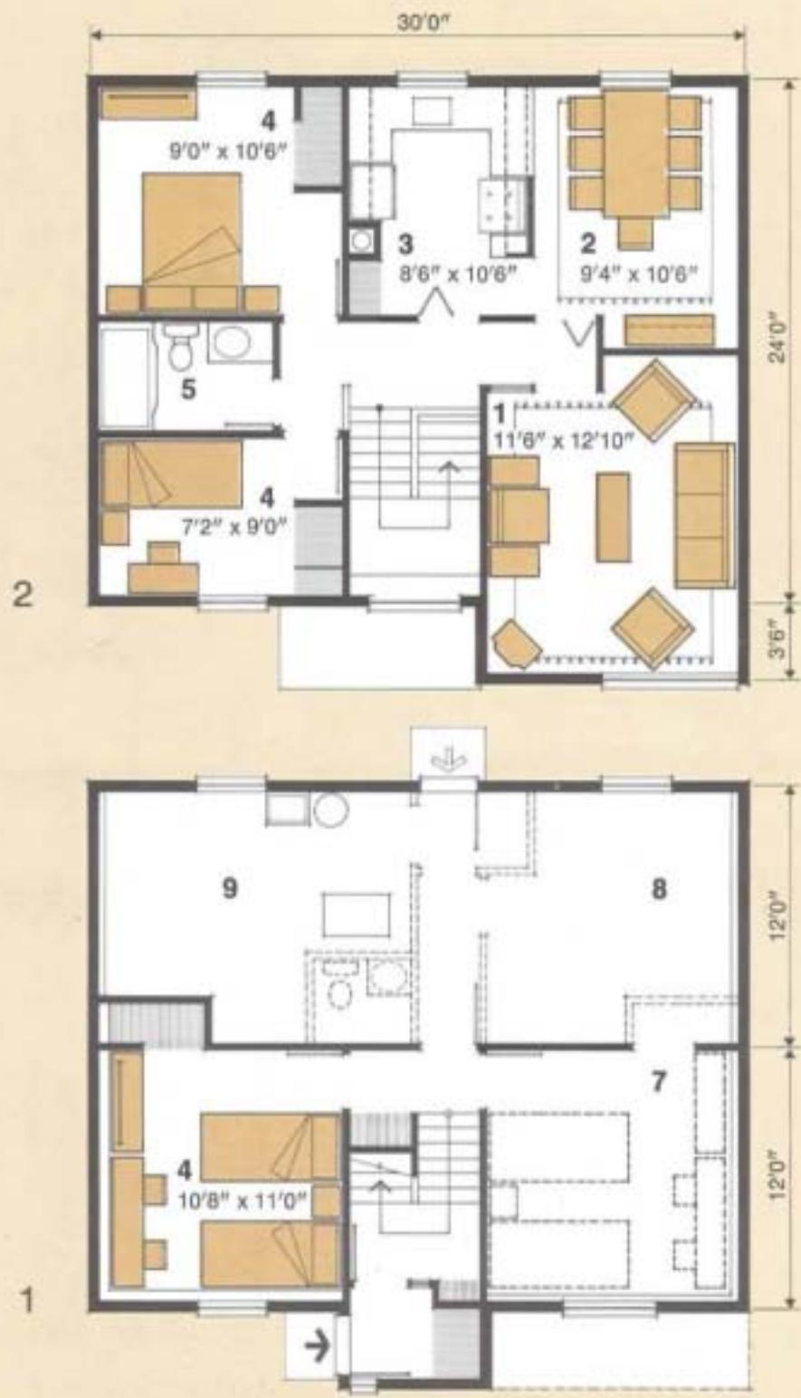
This two-bedroom version of a bilevel house is designed to suit a grade which slopes down from the street on a narrow lot. The narrow side of the house faces the street. The rear entrance is at grade level and as a result, the upper floor circulation is reduced to a minimum. The third bedroom, which is shown completed on the lower floor, need not be included if it is not required initially.
