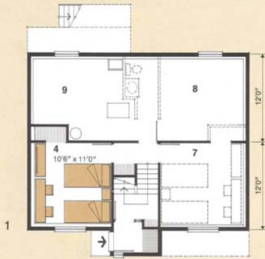
This is a two-bedroom bilevel design. It is intended for a narrow, flat lot with the narrow side of the house facing the street. The upper floor accommodation complies with the requirements of the Residential Standards because both bedrooms are adequate in size. As a result, the third bedroom which is shown as completed on the lower floor need not be included if not required immediately. The upper floor circulation provides clear separation between the bedroom area and the rest of the house.
