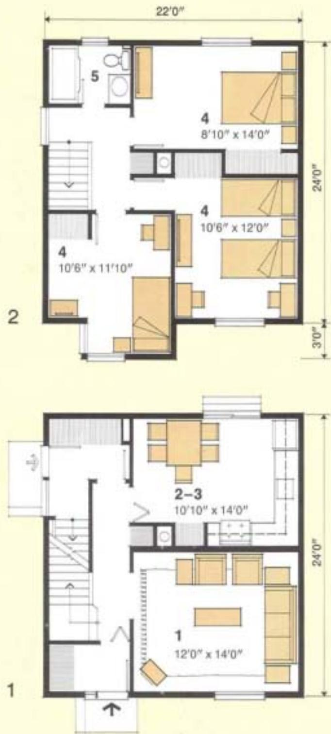
This three-bedroom, basementless, two-storey house is designed for siting on a narrow lot or a gently sloping one where the presence of rock would preclude the use of a basement. The design provides a single-storey addition to the side of the house for heating and storage and locates the laundry part of the utility in the kitchen/dining area. Additional storage space is provided under the stairs. The side entrance has a mudroom to pass through before entering the main part of the house.
