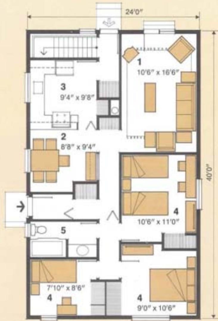
This three-bedroom basementless bungalow is planned primarily for a narrow flat lot with the living room facing the street. The zoning of the house separates the bedrooms on one side from the remaining functions on the other. The utility room at the rear of the house contains the laundry, heating, and storage components all convenient to the secondary entrance and the side yard.
