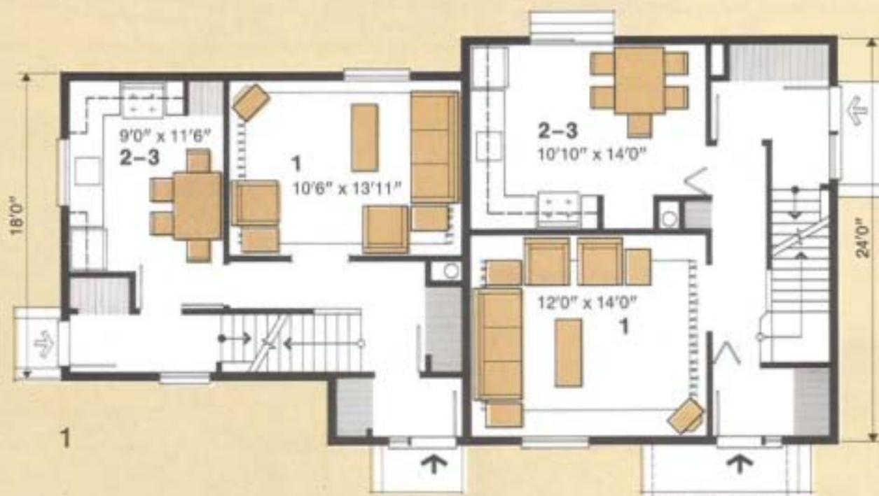
In this composite design, two different bilevel houses are combined. The house on the left is design 1.09 (floor area 1055 sq. ft.) while the house on the right is design 1.10 (floor area 1063 sq. ft.). Both of these designs are illustrated in Part ONE of this book.
