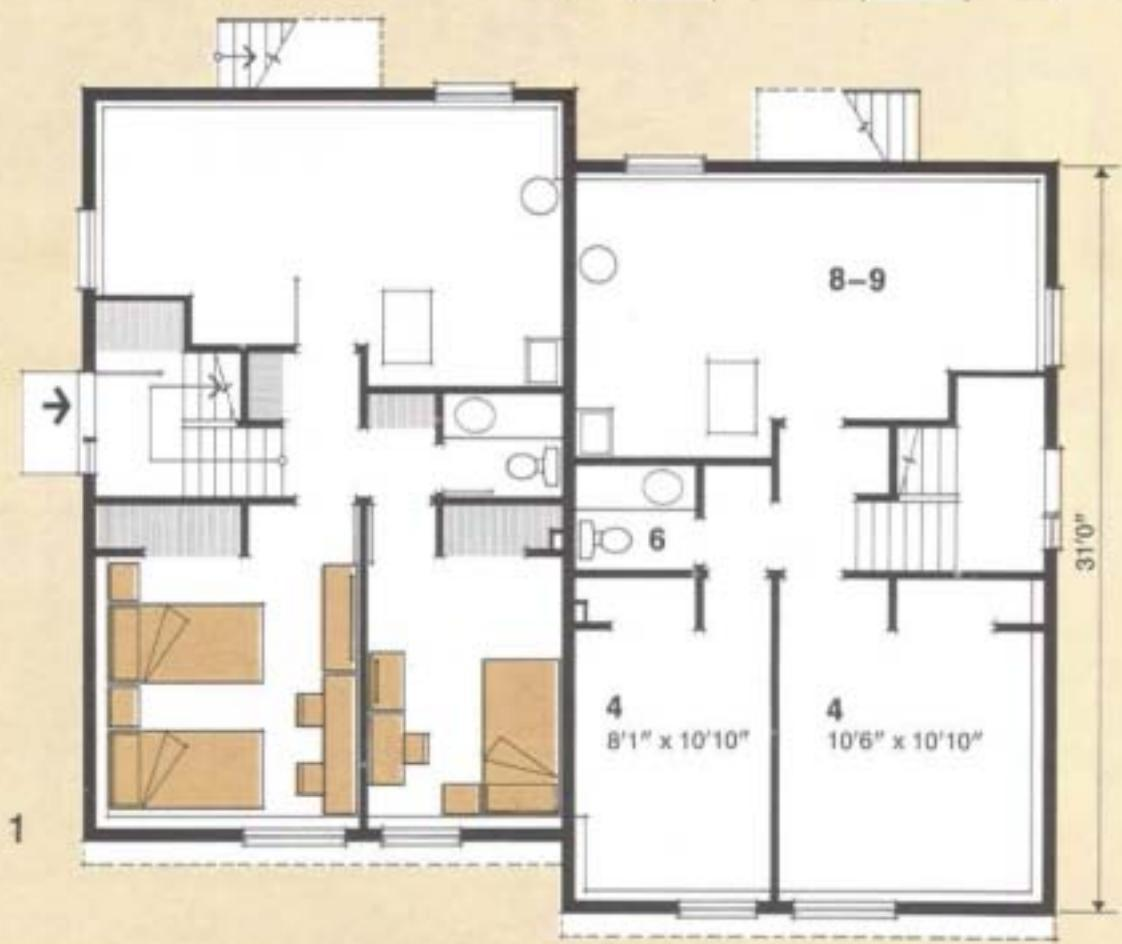
Both of these bilevel houses have the same floor plan as design 1.19 except that in this version, which is more suited to lots which slope up from the street, a direct access to grade is provided from the kitchen/dining area.
