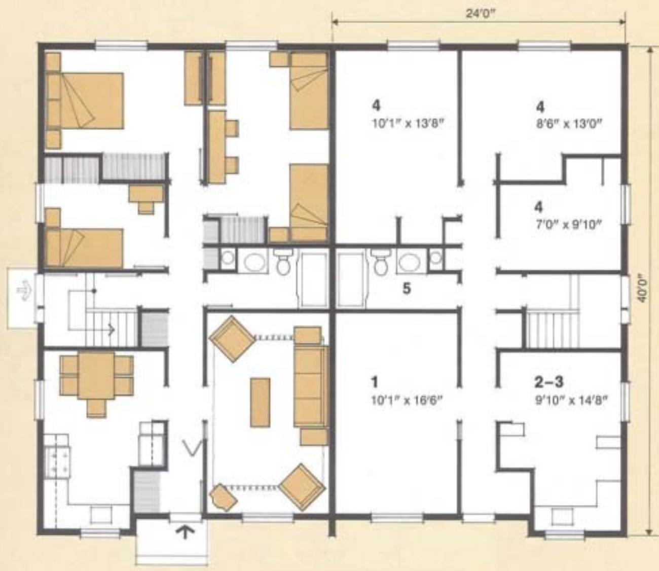
The three-bedroom two-storey house, with basement, which is shown on the left side of this design is similar in plan to the detached design No. 1.08. However, because the utilities, laundry and storage are all located in the basement in this design, the side addition shown in design No. 1.08 is not needed. The right side plan is a mirror version of the plan on the left.
