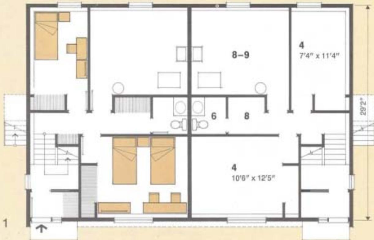
This three-bedroom bilevel design is intended primarily for use on narrow, flat or gently sloping lots. The main entrance is located on the side of the house and the living room and all three bedrooms of each house face the street. The interior circulation has been kept to a minimum in these plans.
