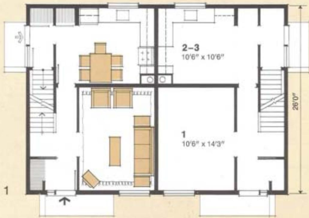
The three-bedroom two-storey house, with basement, which is shown on the left side of this semi-detached design has the same floor plan as the detached design No. 1.07. The house on the right side is a mirror version of the one on the left.
