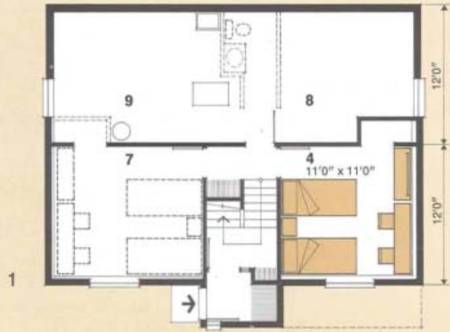
This two-bedroom version of a bilevel house suits a narrow lot which slopes up from the street. There are no windows on the rear wall of the lower floor which permits the grade to be higher on this wall. The third bedroom, which is shown completed on the lower floor, need not be included if not required immediately as both bedrooms on the upper floor comply with Residential Standards.
