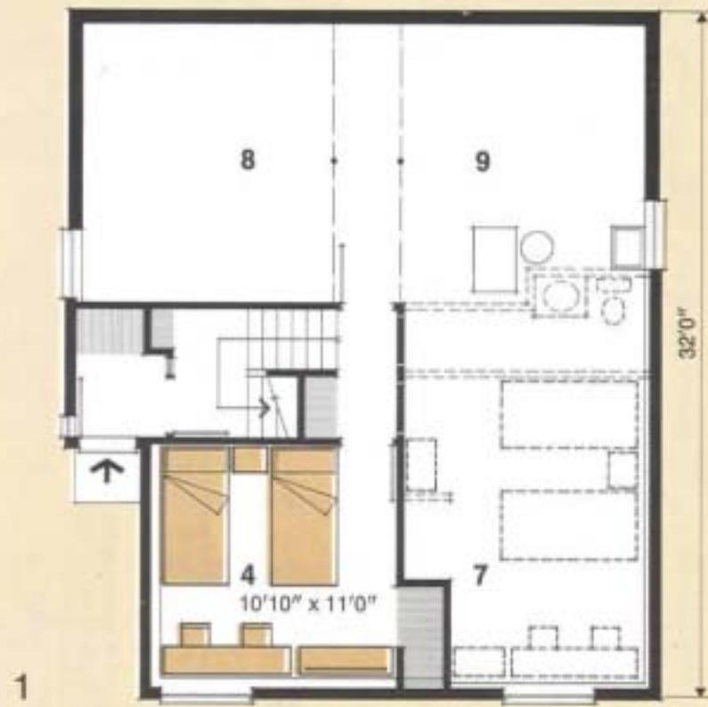
This three-bedroom bilevel house is suitable for a lot grade which slopes down from the street and where the house would be sited with the long side facing the street. To take advantage of the slope, the design locates the rear entrance on the lower floor to provide a grade access. This feature reduces the amount of circulation on the upper floor to a minimum. The third bedroom shown completed on the lower floor must be included to make the plan comply with Residential Standards.
