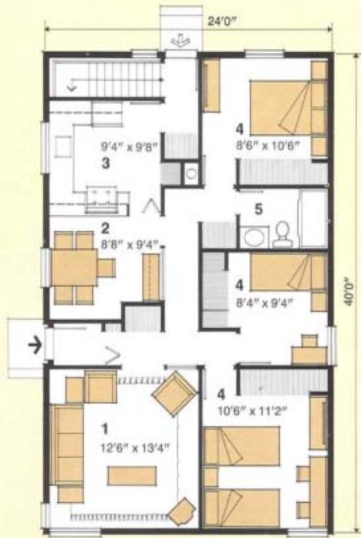
This three-bedroom bungalow, with basement, is primarily for use on a narrow flat lot. The living room, which should face to the south or east, provides direct access to the rear yard. The plan is functionally zoned into sleeping, living, and dining/kitchen areas, with basement access directly from the rear entrance vestibule.
