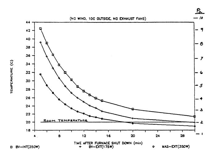
FIGURE 2: Mean Flue Gas Temperature Decay (C)
