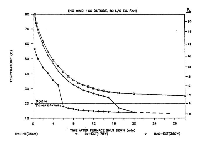
FIGURE 3: Mean Flue Gas Temperature Decay (C)
