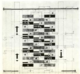
Circulation pattern: Vertical circulation one way up or down. Pedestrian circulation above platform and on the pedestrian street on top. Access circulation interpenetrating the entire complex.
