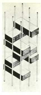
The repetitive spiral stack: box elements span 32 feet and the services are located in the central shaft. The stacks can be grouped in several ways.
