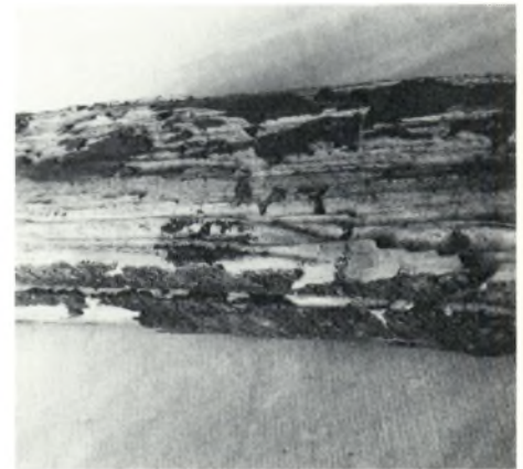
Subterranean termites have attacked this piece of buried wood causing extensive damage to it.
