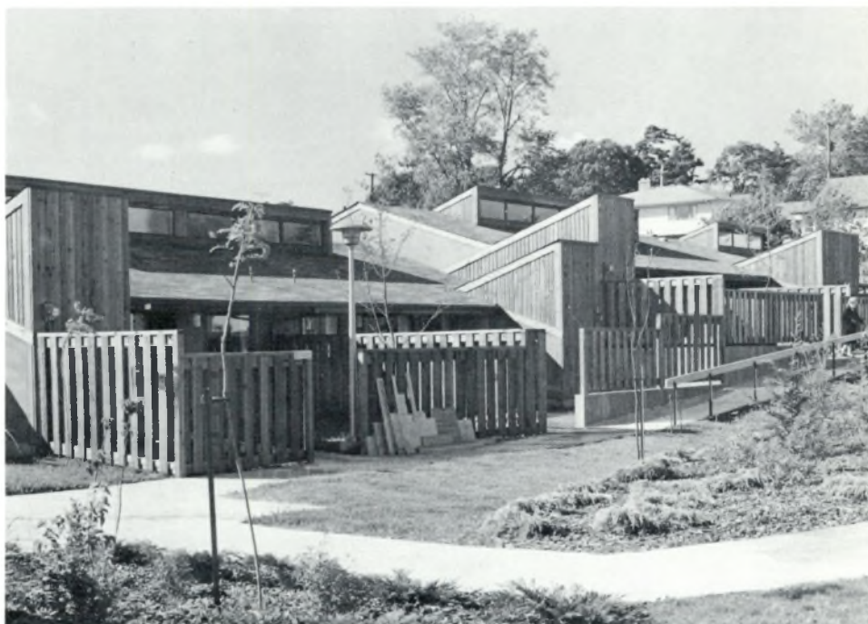
The first two floors of the apartment building, and the townhouses, are provided with ramped access and easily 'navigable' sidewalks for wheelchair users.
