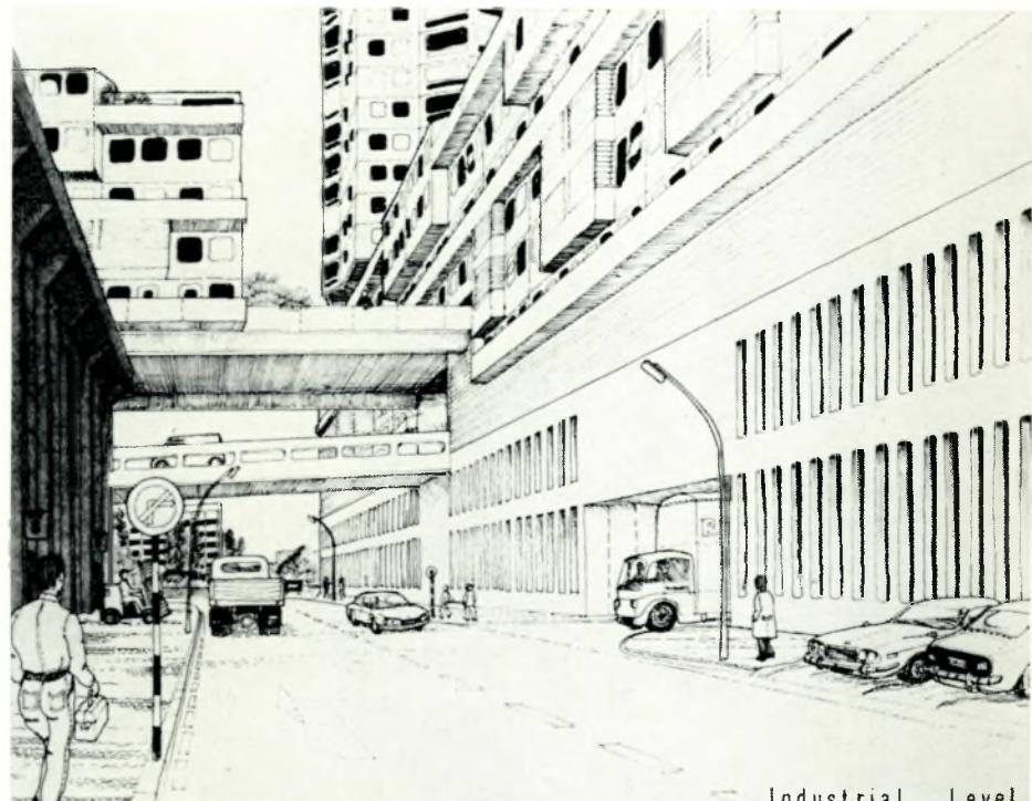
*Artist's impression showing the low-rise and high-rise housing blocks growing up from the roofs of the factories at ground level. There are three roadway systems, one serving the factories, one giving access to the housing schemes, and one above that for pedestrians.*
