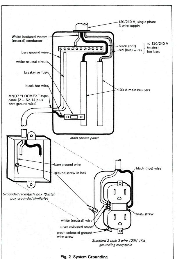
equipment plugged into this receptacle will then be energized at full line voltage (120 V). This occurs because the green grounding conductor in the line cord connects the case and plug, causing a very hazardous situation.
