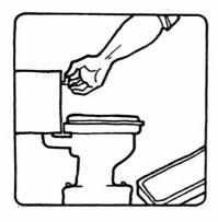
Flush the tank once to dislodge water from the flushing channels of the toilet bowl. The antifreeze will collect in the trap.
