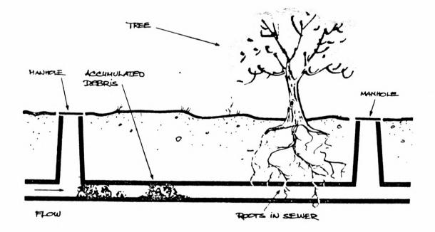
Figure 10 Sewer Blockage
