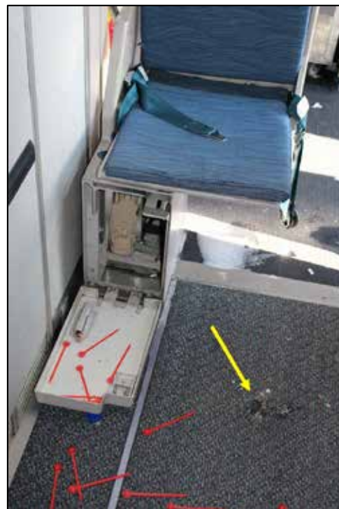
Figure 12. Floor damage above FR65
