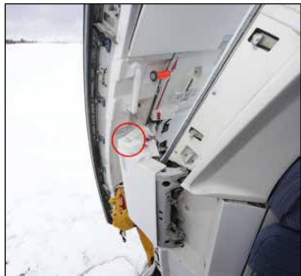
Figure 5. Gust lock release pushbutton (circled) on the L1 door
