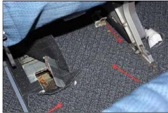
Figure 11. Floor damage forward of passenger seat 33D
