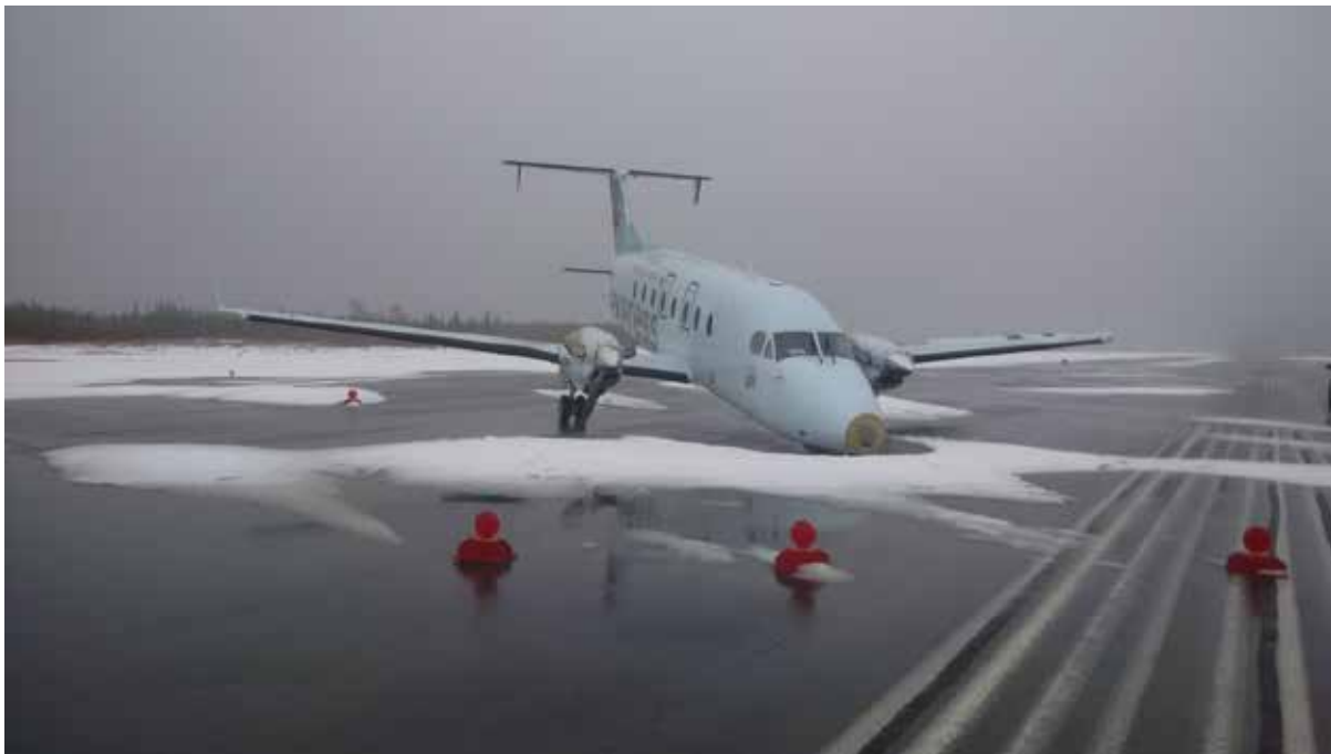
Figure 2. C-FEVA on the day after the occurrence showing the nose landing gear collapse
