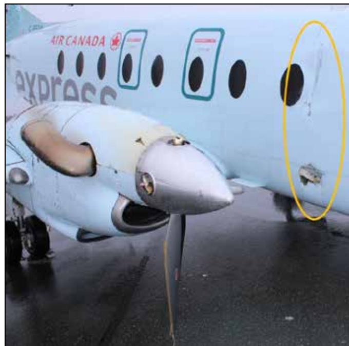
Figure 4. Fuselage with damage caused by propeller blade (circled)
