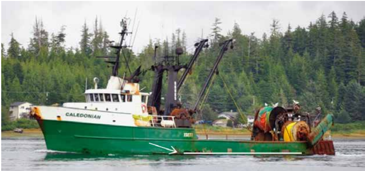
Photo 4. Caledonian in loaded condition. The white line on the hull indicates the estimated level of the vessel's working deck (Source: Eric Sorenson, with TSB annotations)
