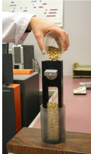
NIR sample cell for whole grain
