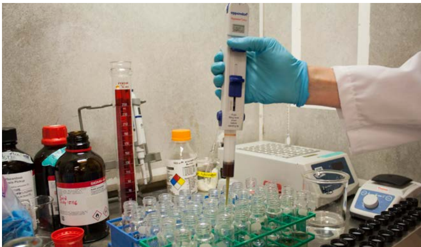
Determination of arabinoxylan content in barley by gas chromatography (GC) involves acid hydrolysis of the polymers to arabinose and xylose, derivatization of sugars to corresponding alditol acetates (Top photo), followed by separation and quantification by GC with flame ionization detector (FID) (Right photo).
