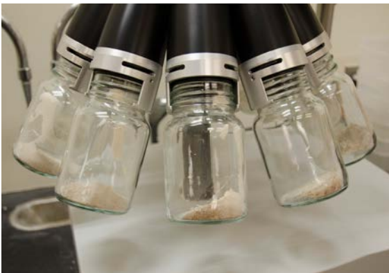
Dividing ground oats for mycotoxin analysis (above and right). Mycotoxins are not evenly distributed in oat kernels and ground oats (far right), therefore systematic methods are used for sample preparation to prevent inaccurate mycotoxin measurements.
