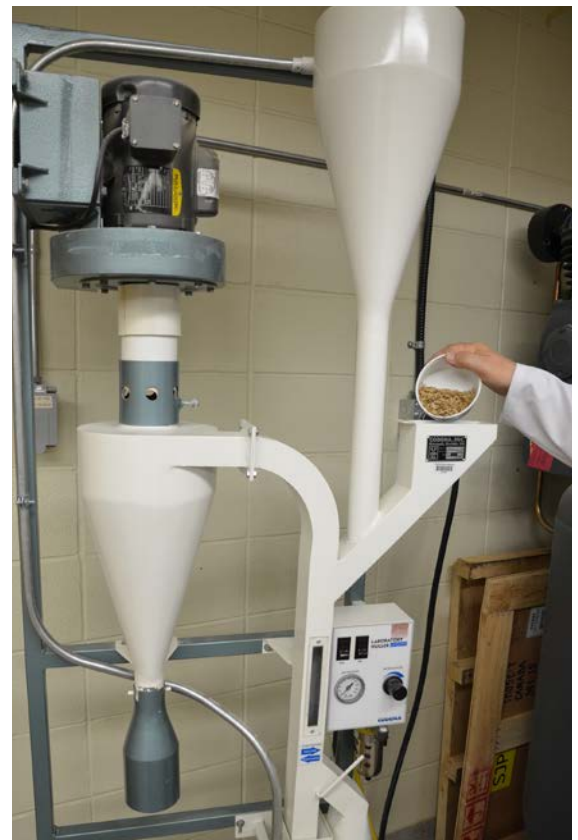
Hulling oats in the Grain Research Laboratory.
