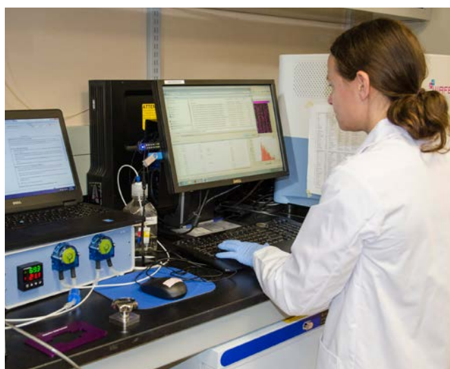
Placing a PCR chip that contains 5,200 nano-reactions into a thermocycler, which is used for generating amplicon pools of DNA barcodes (target enrichment). The DNA barcodes are sequenced by Next Generation Sequencing (NGS) and used in metagenomic analyses for microbial population studies.
