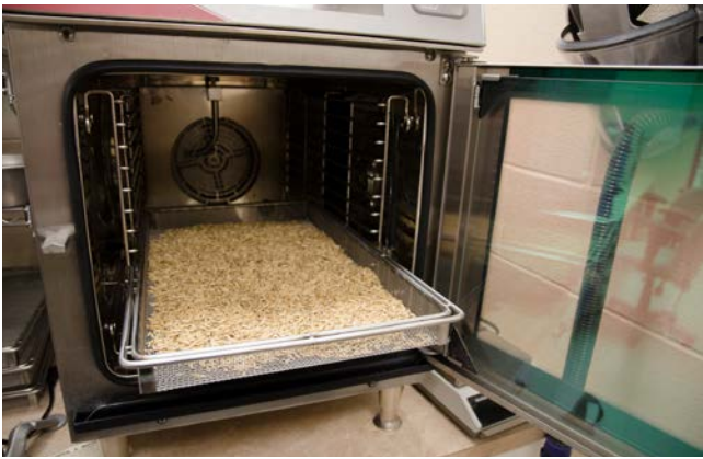
Heating oats in an oven. The effects of heat treatment on mycotoxin concentrations is being studied.
