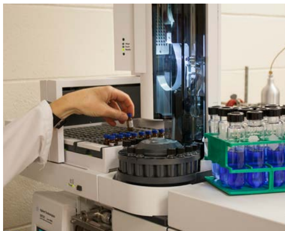
Determination of arabinoxylan content in barley by gas chromatography (GC) involves acid hydrolysis of the polymers to arabinose and xylose, derivatization of sugars to corresponding alditol acetates (Top photo), followed by separation and quantification by GC with flame ionization detector (FID) (Right photo).
