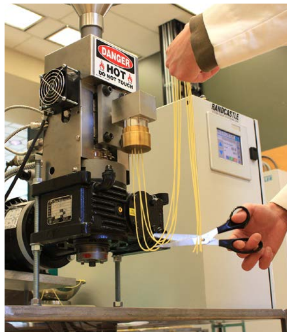
Micro-extruder used for making spaghetti for quality evaluation.
