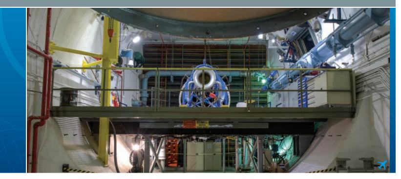
NRC offers a number of gas turbine engine test cells to support performance, operability and certification testing, including icing, bird-ingestion, blade-off, alternative fuel certification, and endurance trials.
