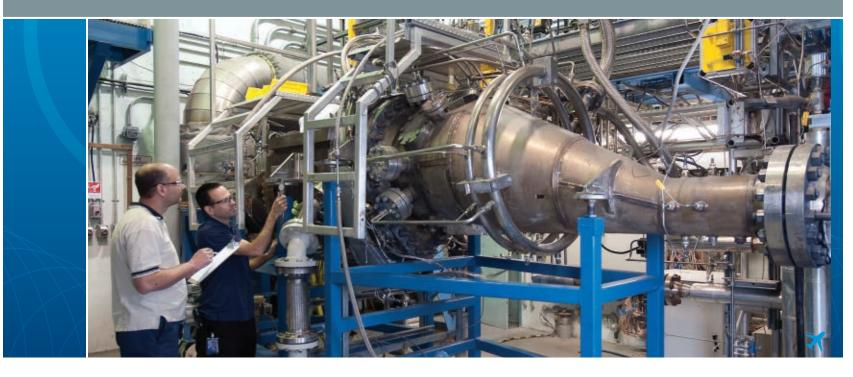
NRC has a multitude of combustion and spray test facilities to support the research, testing and validation of low-emission, fuel-flexible combustion systems, as well as fuel spray nozzles and injectors at realistic high-pressure conditions.
