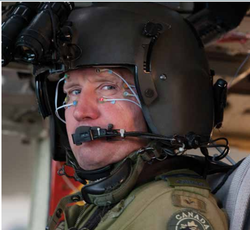
As part of a project on aircrew workload analysis, NRC used electrooculography sensors to capture pilot eye movements.
