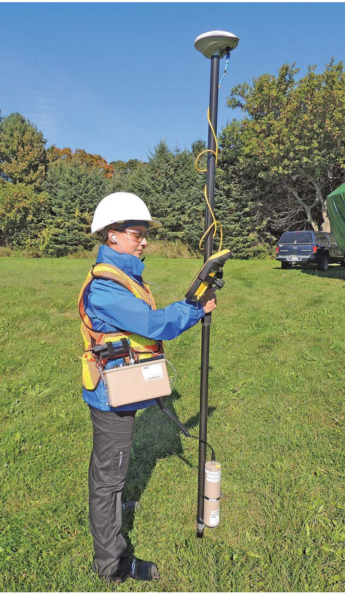
Left: Workers are conducting gamma testing as part of the Port Hope Area Initiative, a large-scale cleanup and safe management of historic low-level radioactive waste initiative in the municipalities of Port Hope and Clarington, in Ontario.
