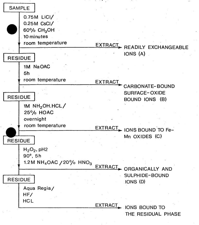
Fig. 1 Outline of the Sequential Chemical Extraction Procedure.
