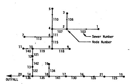
Figure 3 Schematized sewer system layout for pressurized flow routing
