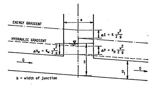
Figure 1 Notation sketch for junction manhole
