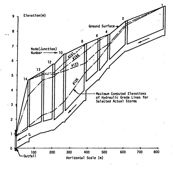
Figure 4 Hydraulic grade lines in a surcharged drainage system
