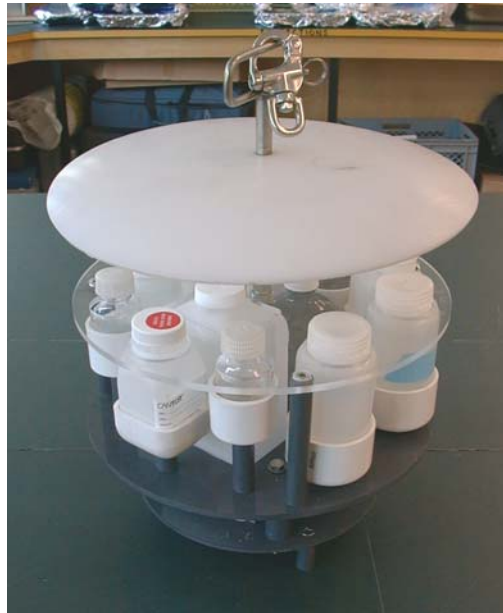
Photo 1 - THE ASSEMBLED MULTI-SAMPLER
