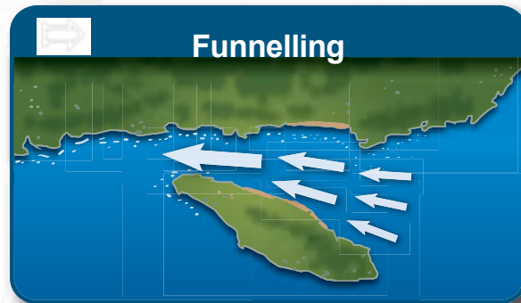
Figure 2o – When wind flows through a narrow opening in the land, its speed is altered but not its direction.
