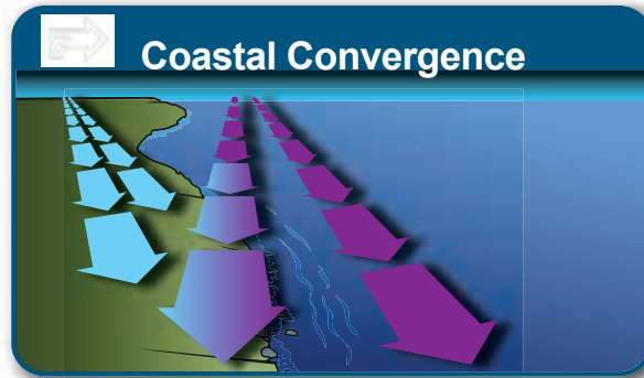
Figure 2l – When the shoreline is to the right of the prevailing wind direction, the wind over the land and the wind over the water will collide, creating a band of stronger winds just offshore.
