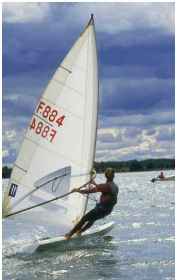
Figure 1c-2 – The force on a sail is a function of the square of the wind speed, making sudden bursts of wind on the water particularly dangerous for sailboats and sailboards.
