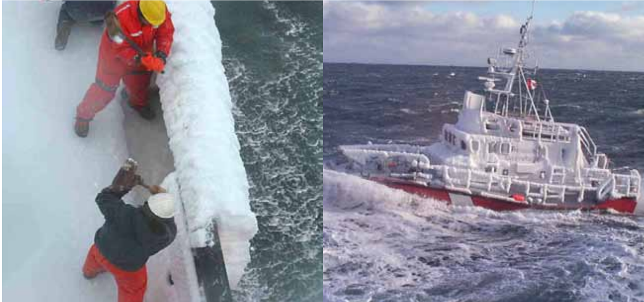
Figure 6a – In cold, wet conditions, a thick layer of ice can build up on the surface of a vessel's decks and rigging, causing a variety of operational problems. Photos : Canadian Coast Guard.
