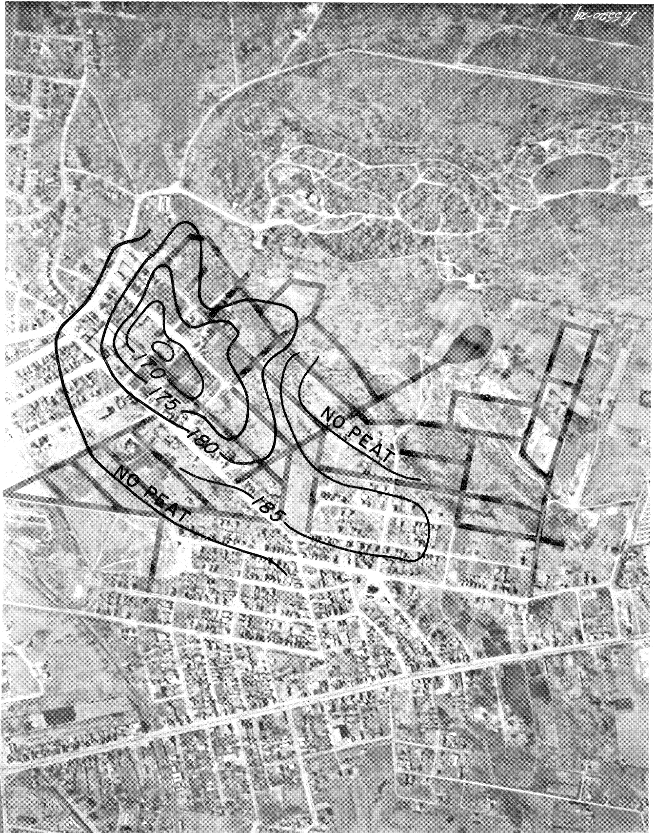
Figure 4: Vertical air photo of part of the city of Vanier Ontario taken in the 1940's. Superimposed are contours in feet above sea level of the solid ground underlying a bog. The grey grid pattern shows streets built since the photograph was taken.
