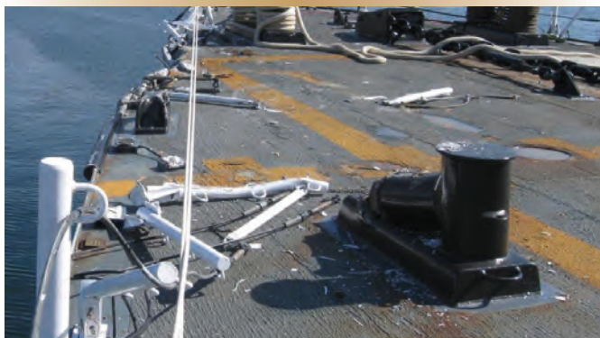
Damage in the immediate aftermath of the allision (left); internal view of bow damage with insulation removed (right).
