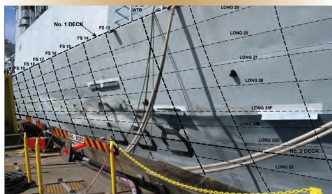
Damage sustained to HMCS Winnipeg 's bow (left); Starboard midship damage caused by Winnipeg coming into contact with the jetty (right). Lines denote location of transverse and longitudinal frames.
