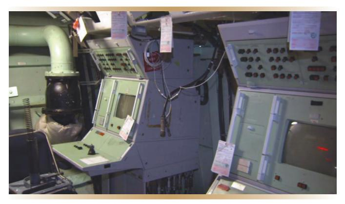
Tags used to identify parts being removed from legacy ships
