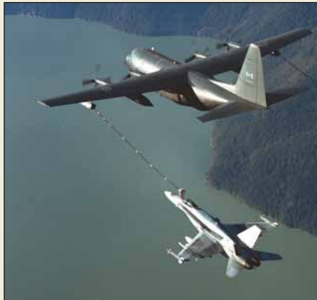
A CC-130 Hercules tactical refueller from 17 Wing Winnipeg's 435 Transport Squadron refuels a CF-18 over Vancouver Island. The CC-150 Polaris's new strategic refuelling capability will permit CF-18s to fly longer distances without landing to refuel.
