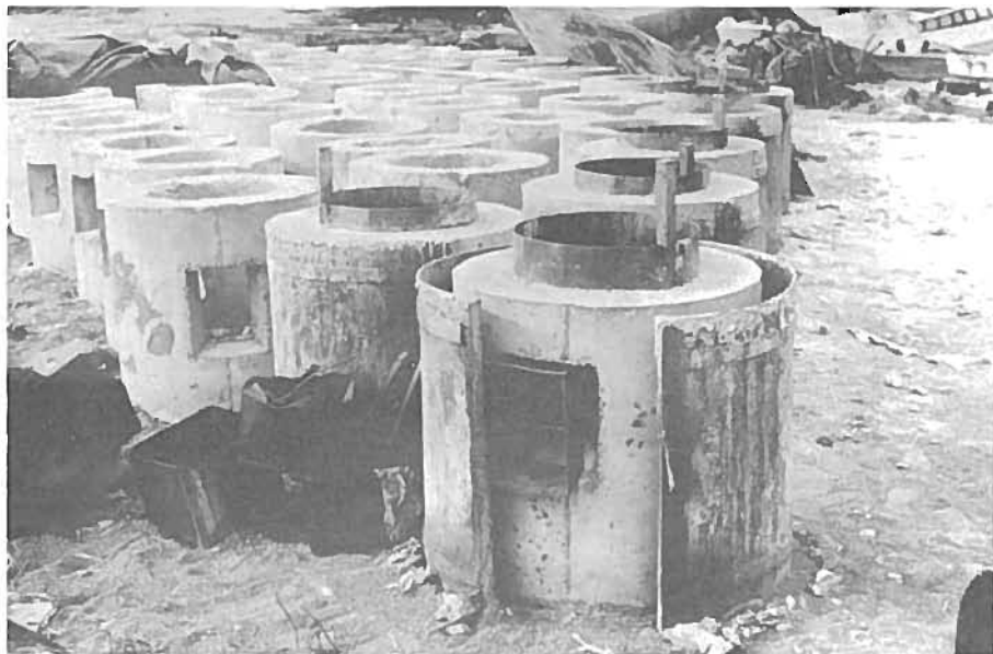
Plate 4. Concrete "planting stones" for Laminaria and moulds of metal and wood used in their manufacture. Usu, Hokkaido. Oct., 1966.
