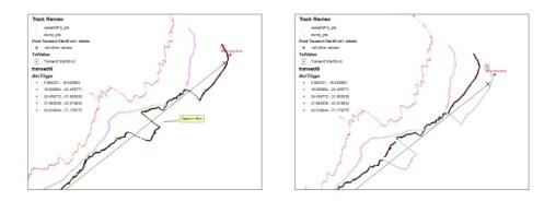
Appendix Figure A. Example 1 of offset error (left) and corrected trackline (right)
