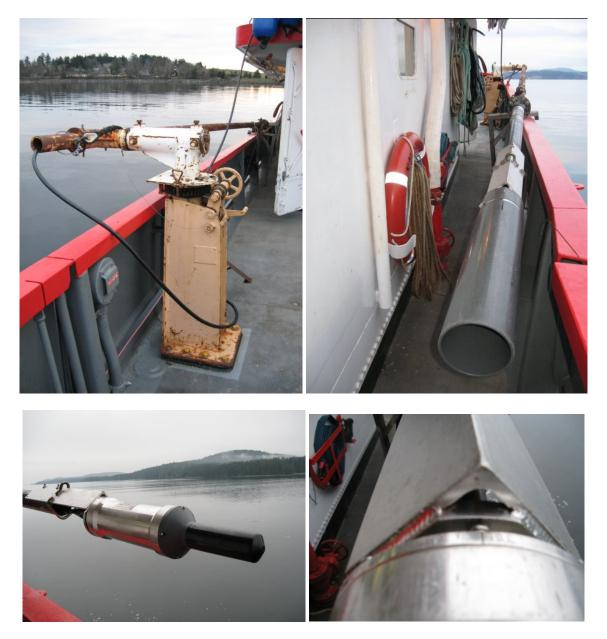
Care of the hydrophone: there are 2 o-rings that should be examined before connecting to the cable. One is located just inside the hydrophone and the other on the outside. The o-ring lubrication for this unit is 'unique'. Use Parker O Lube by Parker Seals or Barium grease. Ensure that no lubrication gets on to the sensor (the black end of the hydrophone).
