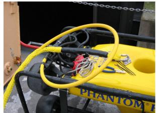
The woven strain relief is looped at one end and a quick link attaches it to the ROV.
