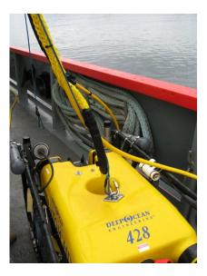
The photo above shows the woven strain relief (here the lift line is attached using loosely fitted zap straps), the lift line (blue rope), and a quick link.
