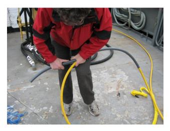
As can be seen in the photo, the woven strain relief is in place and will cover a portion of the hose/umbilical.
