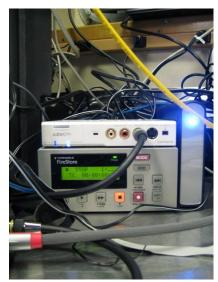
Method #1 - a 3-unit stack consisting of an analog to digital converter, a FireStore hard-drive recorder, and hard-drive. Each unit has its own power supply.
