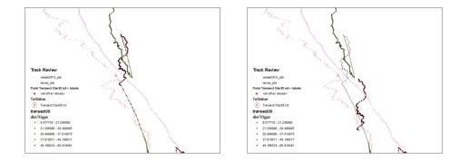
Appendix Figure B. Example 2 of offset error (left) and corrected trackline (right)
