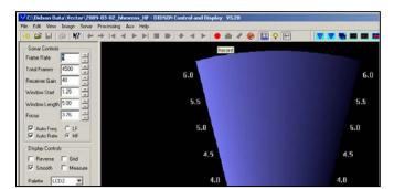
Didson settings: Auto Frequency and Auto Rate should be turned on. Gain should be set at 40. If recording is not staying on, check Image-> Capture ->Record Options -> choose Continuous, then choose N Minutes per file = to 60 or less if short transects.
