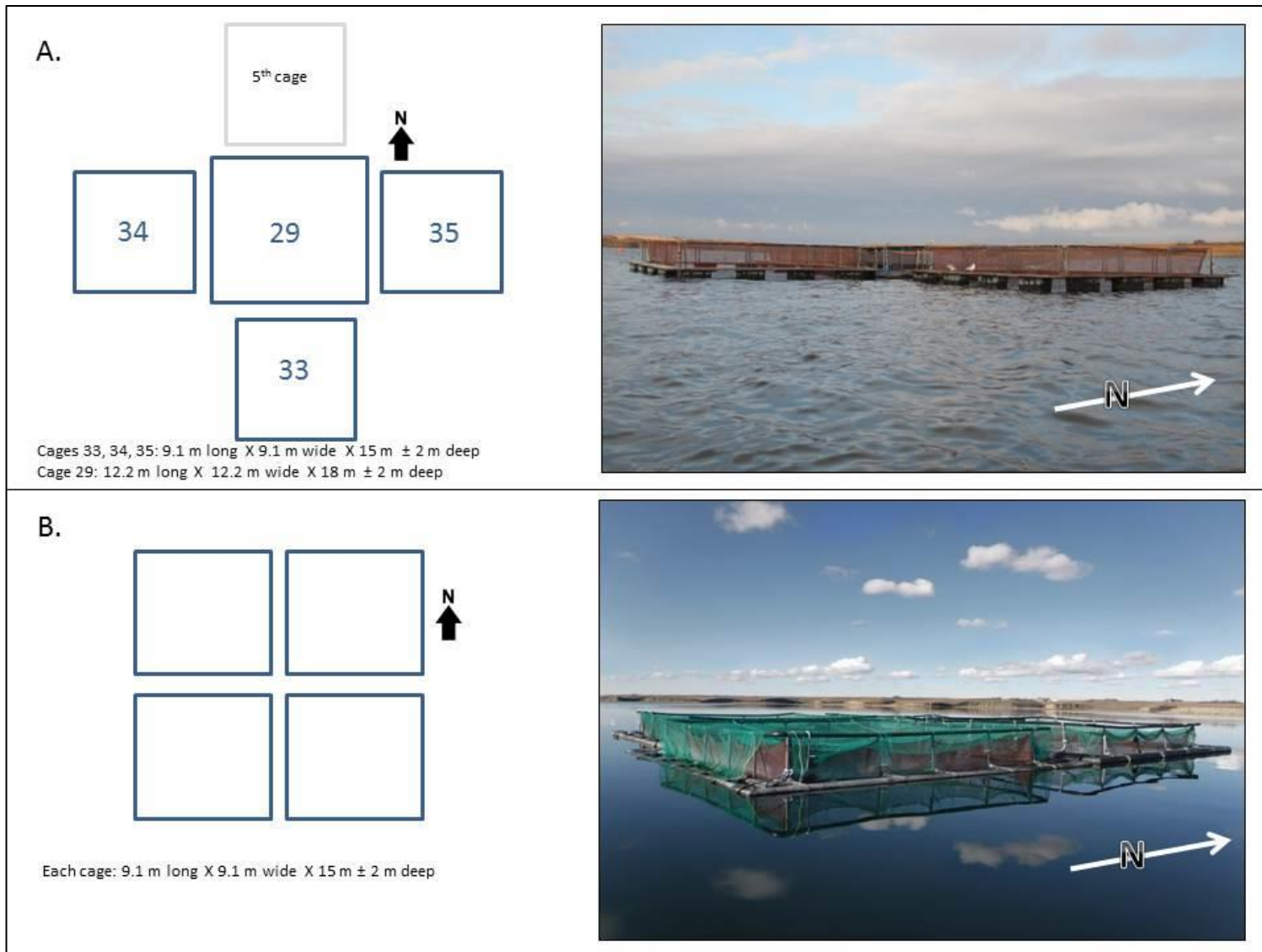
Figure 9. (A) The 2014 and (B) 2015 configuration of Kadla cages with an arrangement of four or five cages in a cross pattern. The 5 th cage was only temporarily installed.
