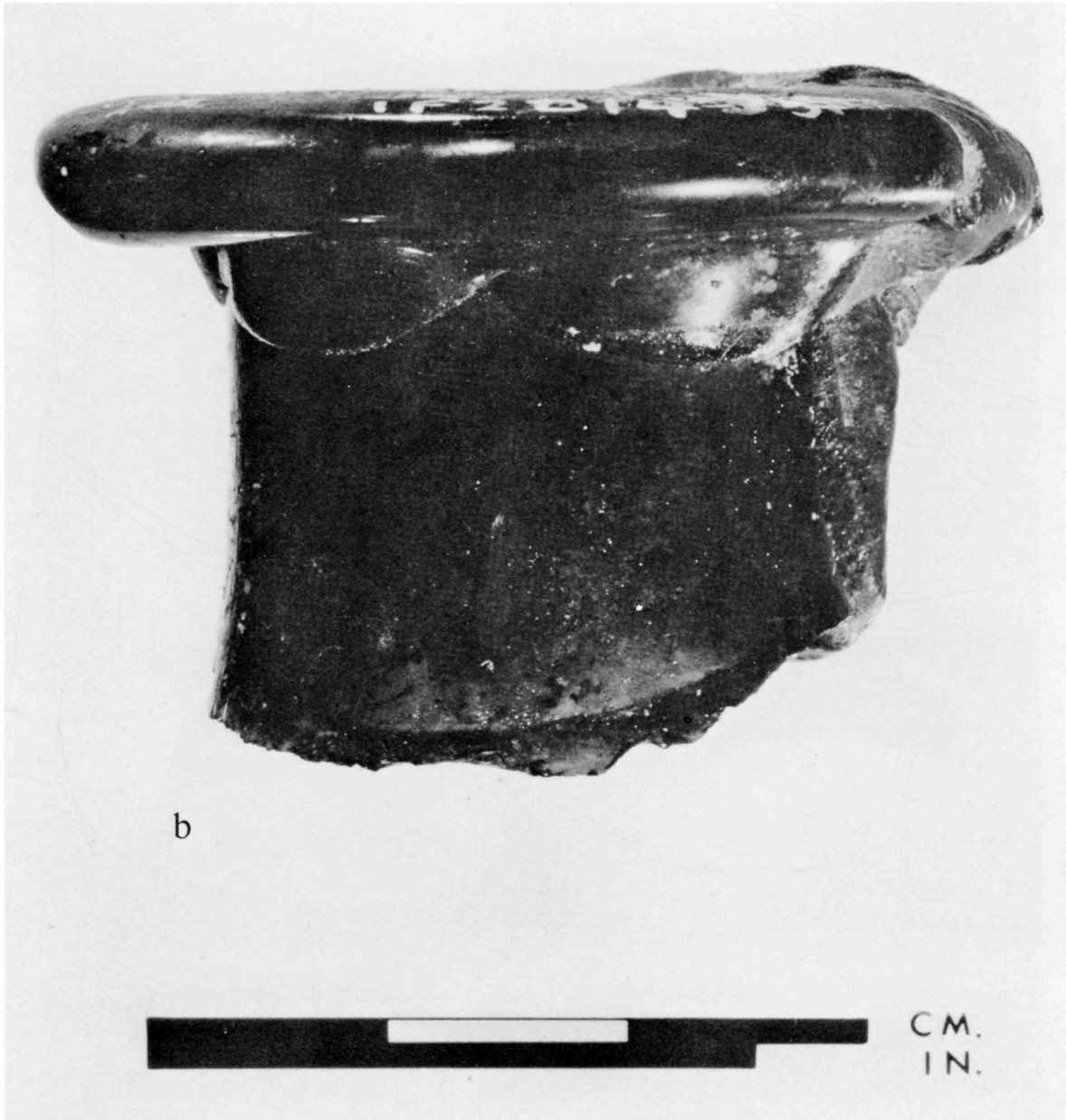
3b Case of gin bottles: neck with hand-made flanged finish.
