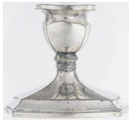
© Government of Canada, Canadian Conservation Institute. CCI 120260-0316 Figure 12: Silver-plated lead candlestick. The dull gray metal where the plating was removed by polishing tested positive for lead.
