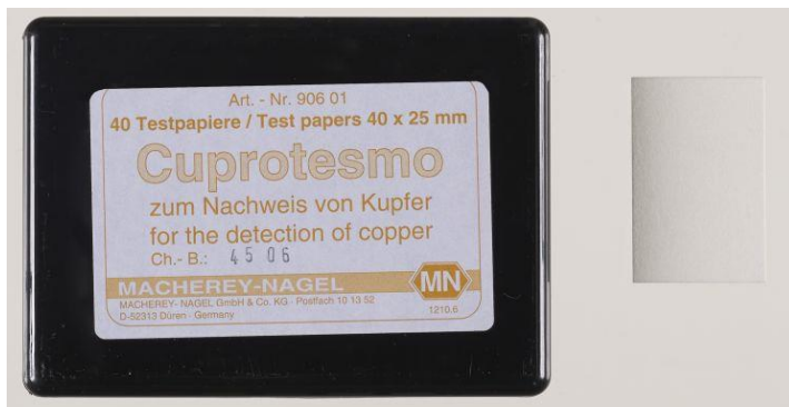
© Government of Canada, Canadian Conservation Institute. CCI 120260-0228 Figure 1: Cuprotesmo test papers. Pictured are the case and a single sheet of test paper.
