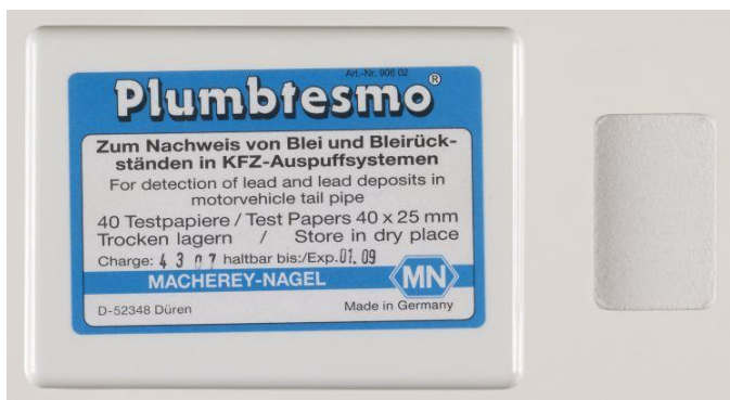
© Government of Canada, Canadian Conservation Institute. CCI 120260-0220 Figure 2: Plumbtesmo test papers. Pictured are the case and a single sheet of test paper.
