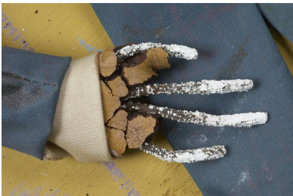
© Government of Canada, Canadian Conservation Institute. CCI 97852-0006 Figure 11: White lead corrosion on armature wire for a puppet's hand.
