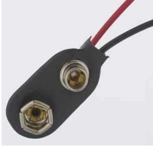
© Government of Canada, Canadian Conservation Institute. CCI 120260-0247 Figure 14: Battery snap for a 9-volt battery.
