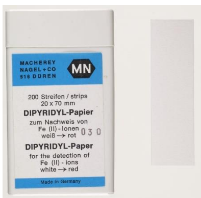
© Government of Canada, Canadian Conservation Institute. CCI 120260-0234 Figure 2: Macherey-Nagel commercial spot test papers for iron (dipyridyl paper 90725). Pictured are the case and a single sheet of test paper.
