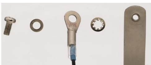
© Government of Canada, Canadian Conservation Institute. CCI 120260-0250 Figure 17: Hardware for attaching ring terminal to threaded hole in tweezers in correct order.
