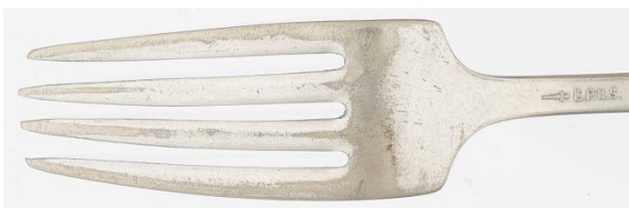
© Government of Canada, Canadian Conservation Institute. CCI 120260-0354 Figure 11: Fork made with a nickel silver alloy and electroplated with silver. The areas where the plating has worn off tested positive for nickel. (The paper turned pink, but there was also a yellow precipitate probably from interference by copper.)
