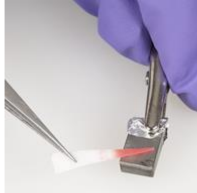
© Government of Canada, Canadian Conservation Institute. CCI 120260-0237 Figure 5: Detail of iron test paper, dipyriddy, reacting and turning pink.
