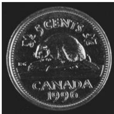
© Government of Canada, Canadian Conservation Institute. CCI 87306-0032 Figure 12: Canadian 5-cent coin made from an alloy containing 75% copper and 25% nickel. The spot test paper turned both pink and yellow (probably interference from copper).
