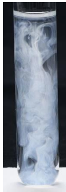
© Government of Canada, Canadian Conservation Institute. CCI 120260-0394 Figure 1b: Test solution showing precipitate of white silver chloride 40 seconds after adding silver nitrate to a solution with a chloride ion concentration of 30 ppm.
