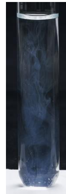
© Government of Canada, Canadian Conservation Institute. CCI 120260-0394 Figure 1c: Test solution showing precipitate of white silver chloride 40 seconds after adding silver nitrate to a solution with a chloride ion concentration of 5 ppm.
