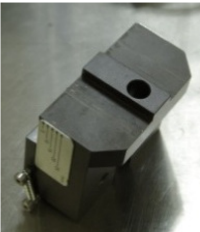
Figure 12: Bottom of the roller support showing bump and bolt hole, bump is needed for good fit into the T-slot.
